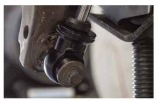
Fig. 13: Install the lower shock bolt (passenger side shown).
