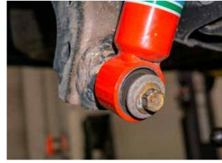
Fig. 11: Remove lower shock mount bolt.
