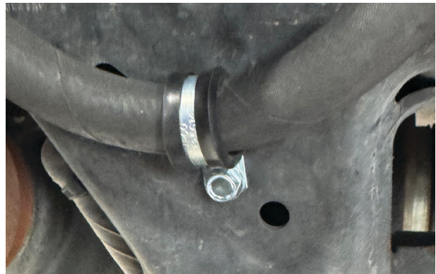
Fig. 29: Install the self-drilling screw.
