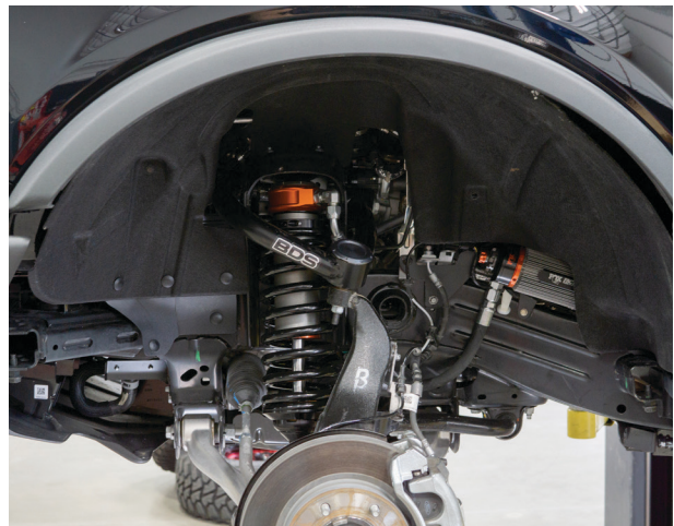
Fig. 30: Trim the fender liner.
