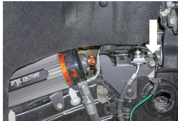
Fig. 24: Install the provided bolt on the passenger side's reservoir bracket.
