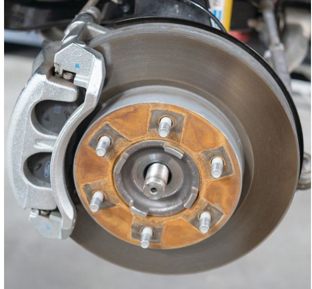
Fig. 5: Push the axle shank flush.
