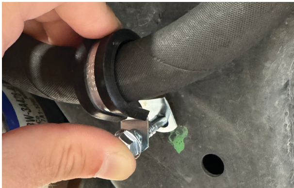
Fig. 28: Position the P-clamp over the hose.
