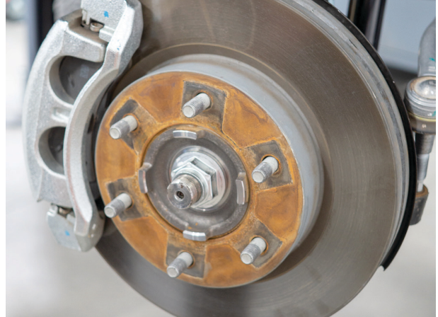
Fig. 15: Fasten the axle nut.
