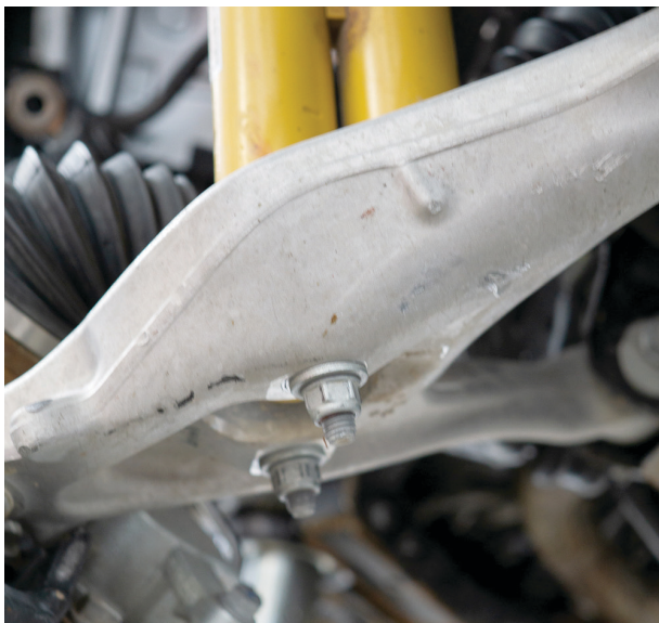
Fig. 9: Take off the bar-pin bolts.
