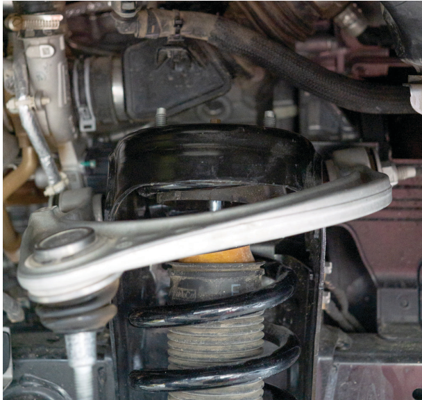
Fig. 7: DO NOT remove the center nut.
