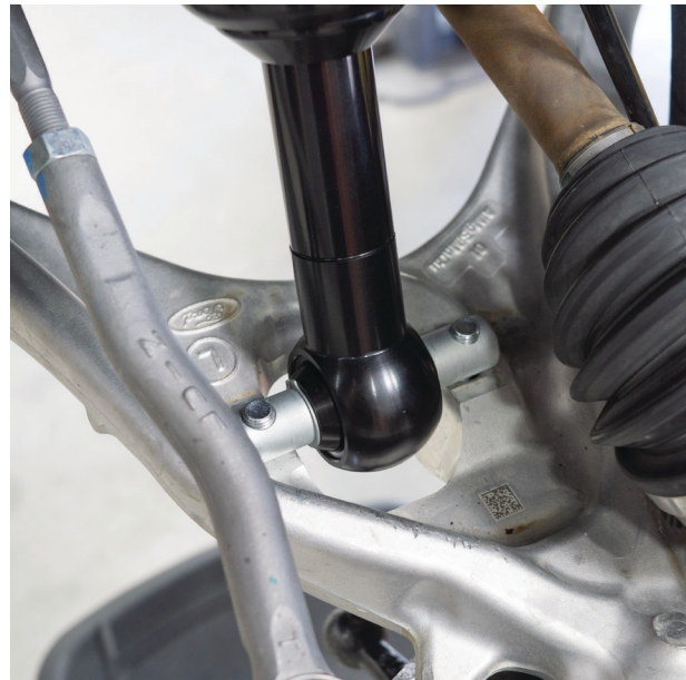
Fig. 13: Fasten the bar-pin bolts.
