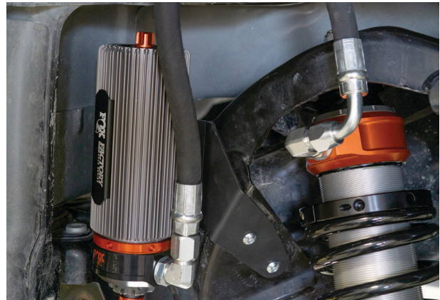
Fig. 44: Mount the reservoir bracket.
