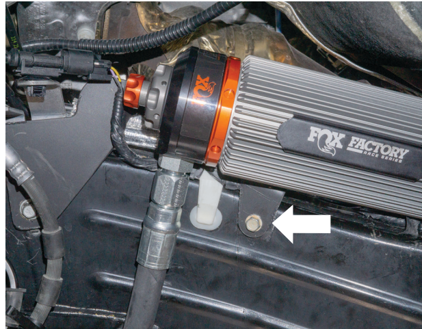
Fig. 27: Install the self-tapping screw.
