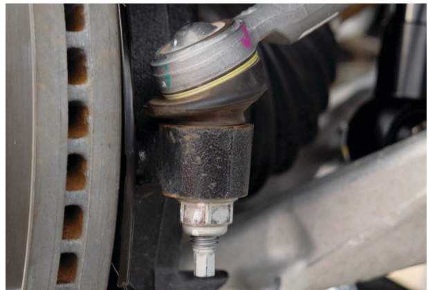
Fig. 16: Tie rod end.
