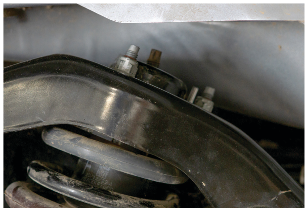
Fig. 34: Do not remove the center nut.
