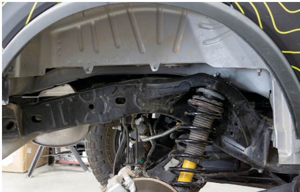
Fig. 31: Pull the fender liner.
