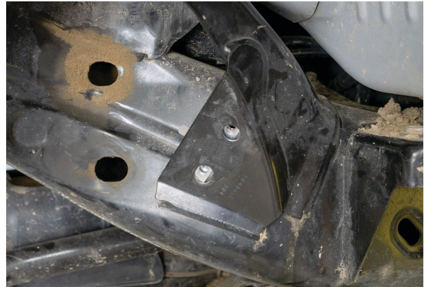
Fig. 42: Locate the backing plate's speed nuts with the holes in the frame.
