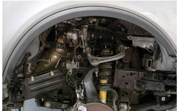
Fig. 1: Pull the fender liner.
