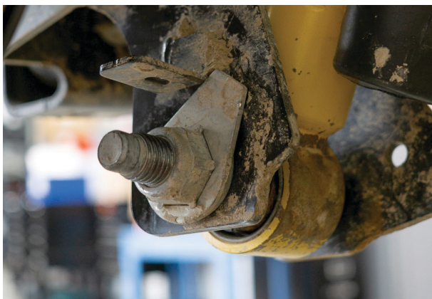
Fig. 33: Loosen the lower mounting bolt.
