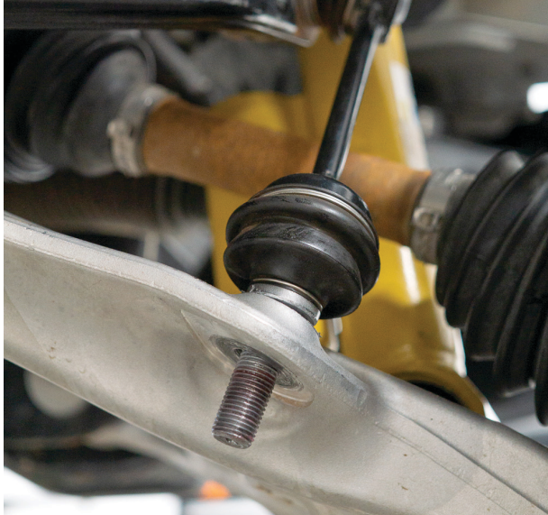
Fig. 4: Disconnect sway bar end link.
