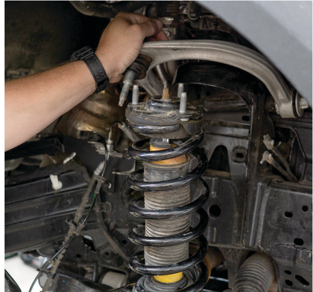
Fig. 8: Free the coil-over from the coil bucket.
