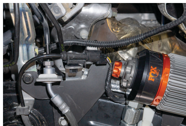
Fig. 26: Fish the ABS wire through the bracket.
