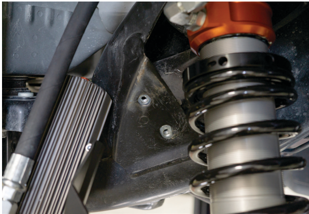
Fig. 43: Align backing plate with the frame.
