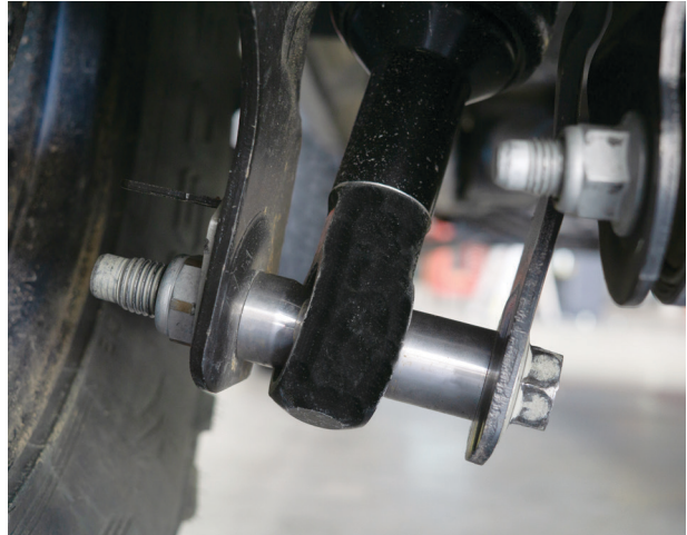
Fig. 38: Note the larger spacer is on the inboard side.
