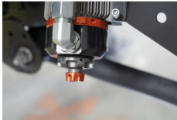
Fig. 22: Mount the reservoir to the bracket.
