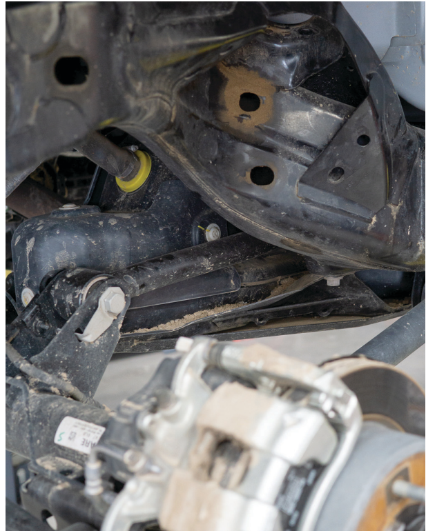
Fig.35: Remove the stock coil-over.
