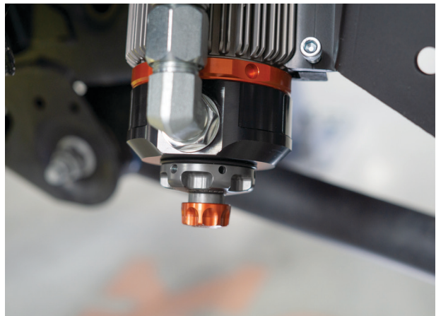
Fig. 40: Mount the reservoir to the bracket.
