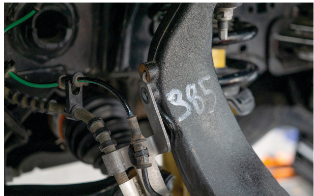
Fig. 2: Disconnect brake line bracket.
