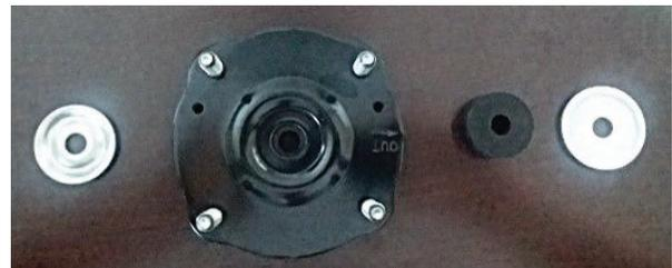
Figure 4: OEM top mount hardware to retain
