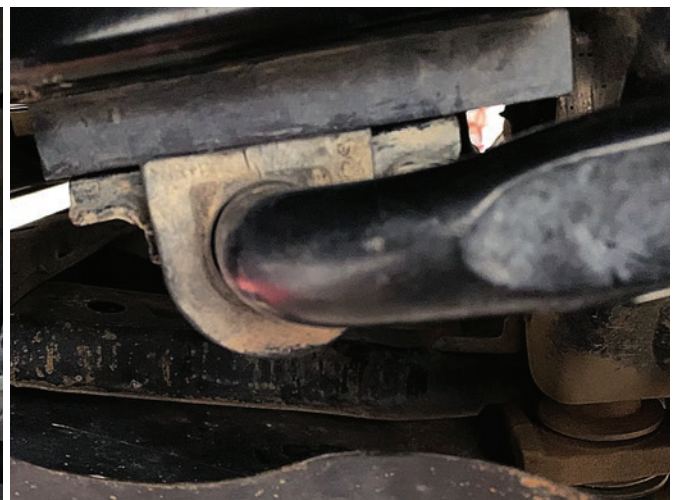
Figure 6: Sway bar relocation spacer (side view)
