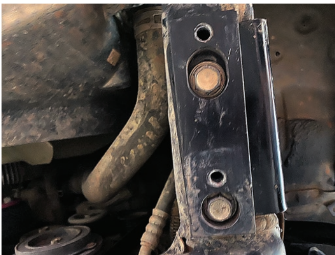
Figure 5: Sway bar relocation spacer (bottom view)
