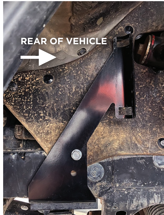
Figure 7: Front reservoir bracket orientation
