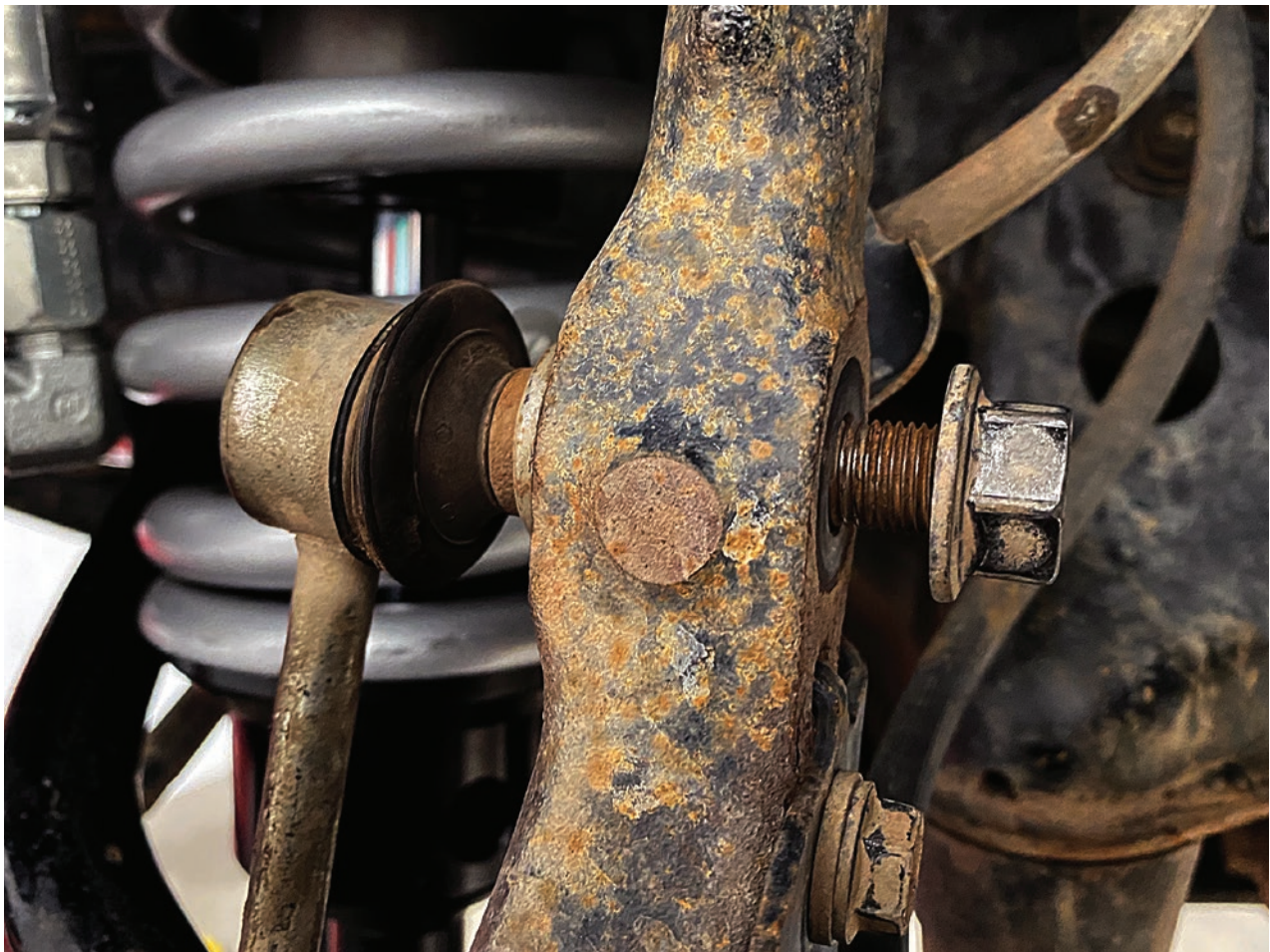
Figure 1: Loosened sway bar bolt
