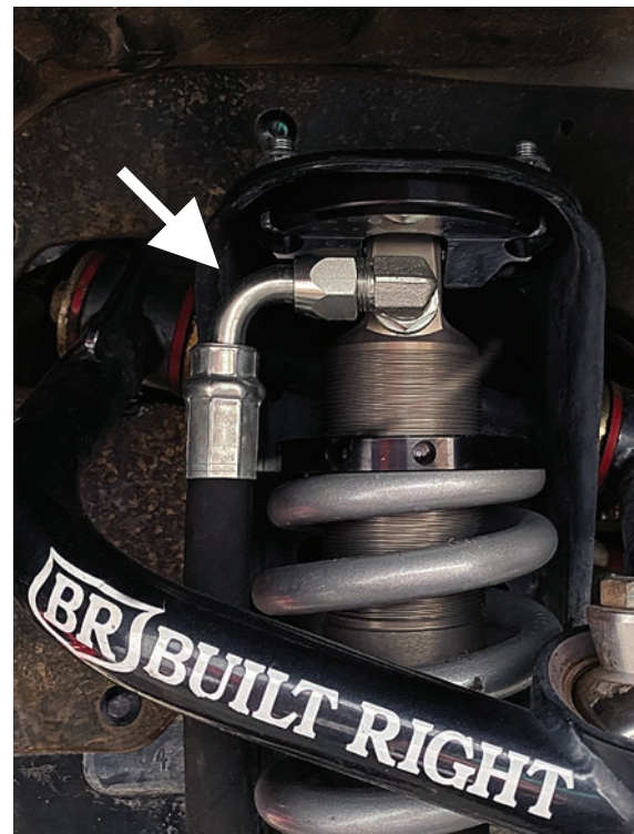
Figure 3: Reservoir hose orientation
