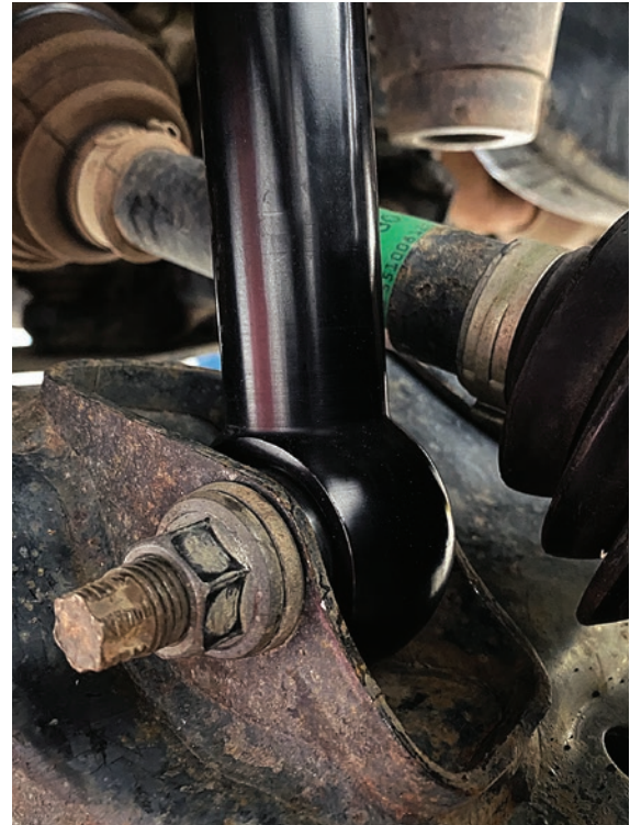
Figure 4: Installed lower shock bolt
