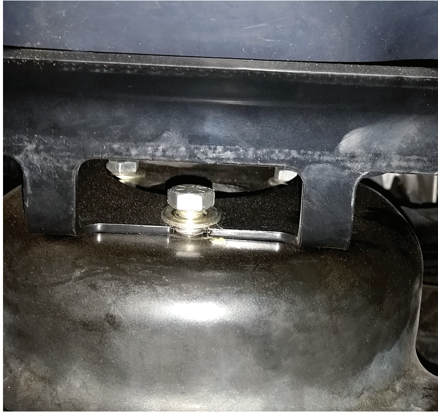
Figure 3: External reservoir mounting bracket
