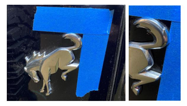
2. Use a heat gun or hair dryer to loosen the adhesive on the back side of the emblem.
