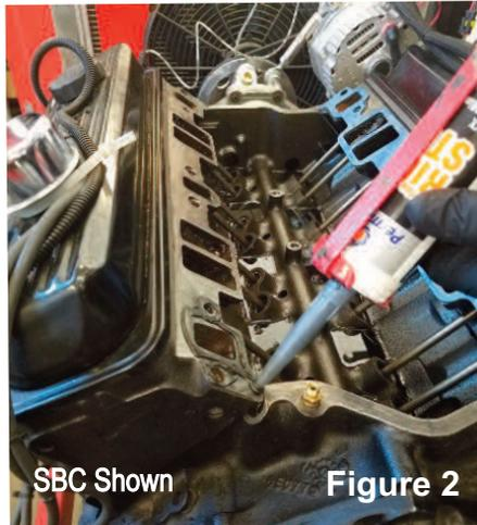
5. Next, lay the intake onto the block and gauge how much silicon will be needed. Apply the proper amount of silicon, proper according to best judgment, to the corners of the valley.
