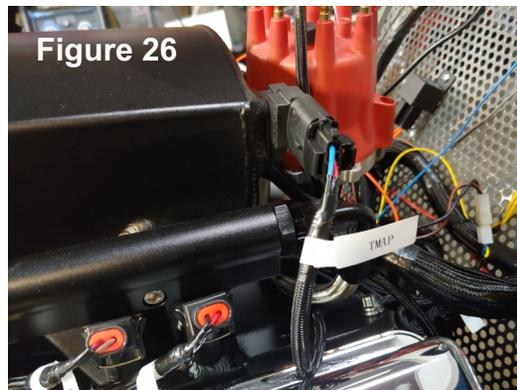
**IAC:** Idle Air Control: Connects on the throttle body
