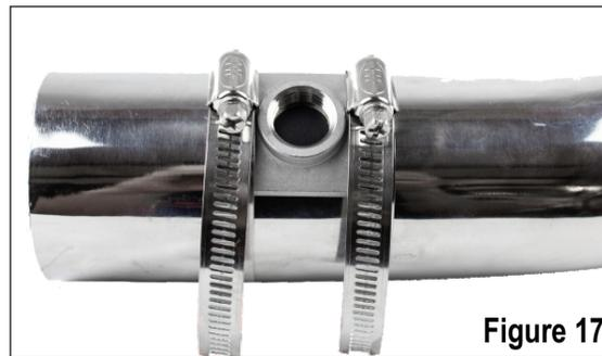
H. Install the sensor into the bung, see figure 18. Apply a small amount of anti-seize on the threads of the O<sub>2</sub> sensor. Be very careful not to get any anti-seize on the tip of the sensor itself because it will cause it to prematurely fail.
