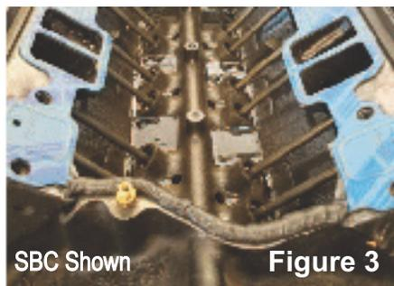
Cover the bridge between the gaskets with silicon to ensure there are no oil leaks.
