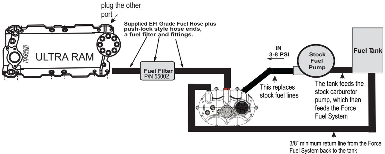
**Go Fuel In-Tank Pump Tank Plumbing Schematic Kit # 50015**
