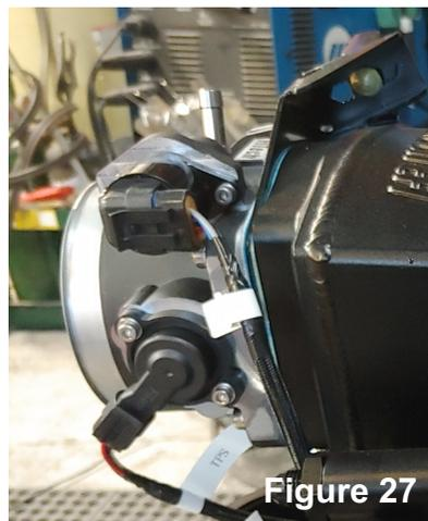
**TPS:** Throttle Position sensor: on throttle body
