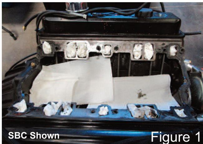
3. Then, lay extra paper towels across the lifters to catch any falling gasket debris through the cleaning process.
