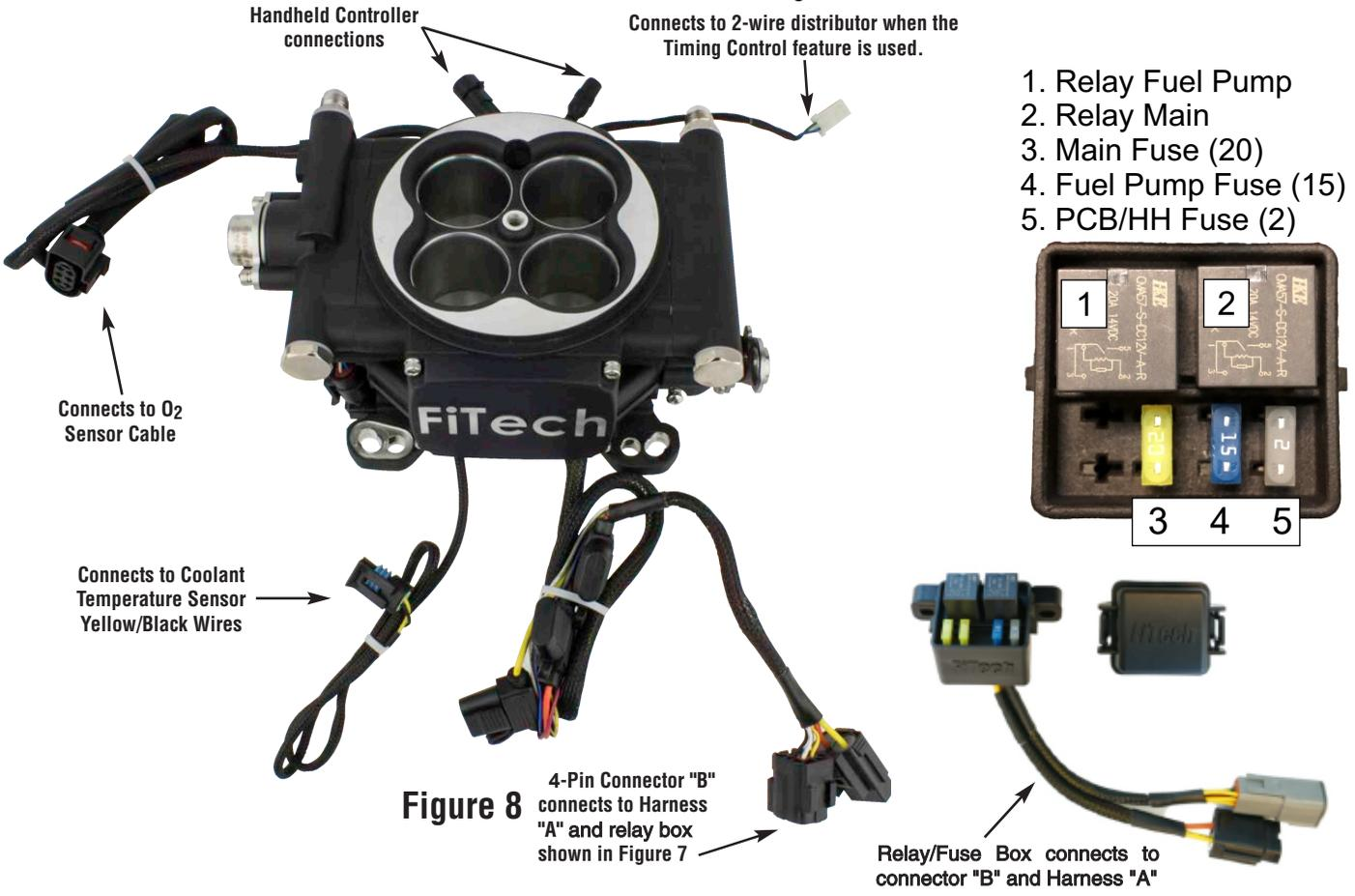
The above photo shows all of the cables that are associated with the FiTech Go EFI System throttle body. The large cable at the bottom left connects to the supplied
