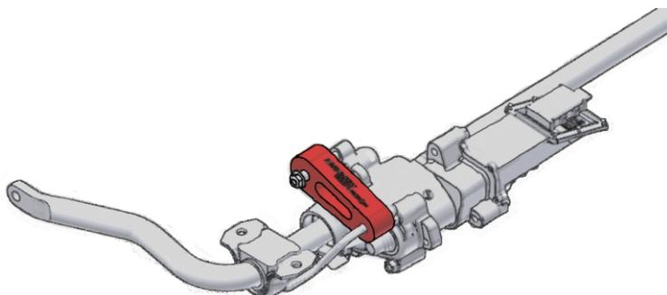
3. Rotate smart bar assembly up into new position.
