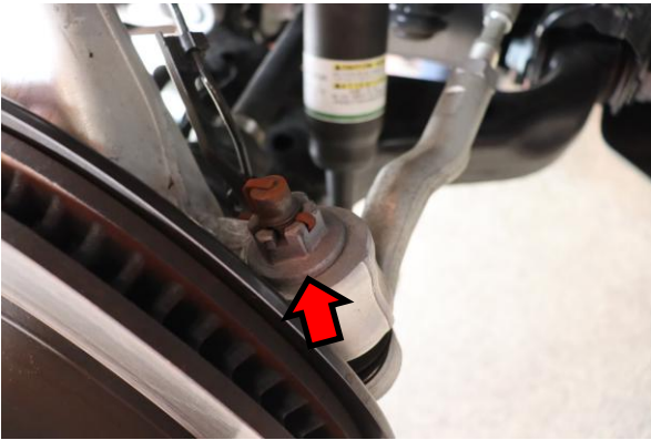
3. Remove the nut from the outer tie rod end ball joint.
