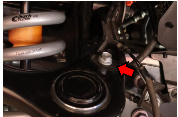
22. Install wheel speed sensor wire harness bracket bolt and tighten to manufacturer specification.
