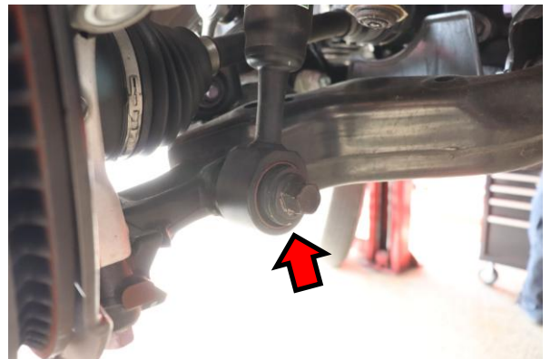
6. Remove the lower shock mounting bolt.
