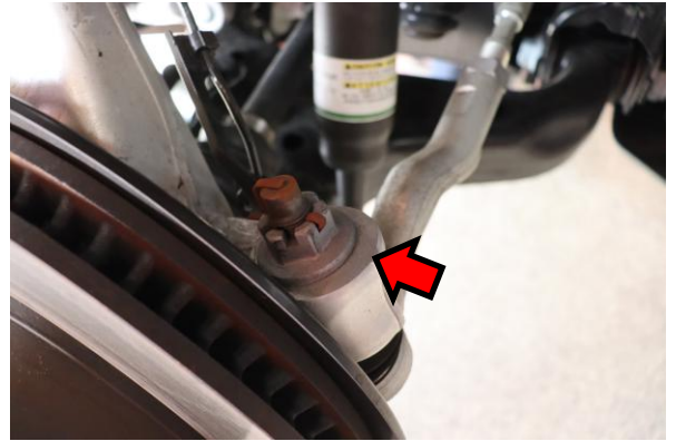
20. Install tie rod end nut and tighten to manufacturer specification.
