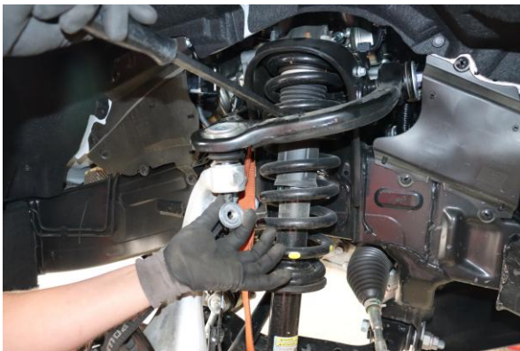
11. Use a pry bar to pull down on the upper control arm and remove the upper control arm ball joint nut. Slowly allow the upper control arm to lift out of the spindle and allow the spindle to rest against the strap installed in step 9.
