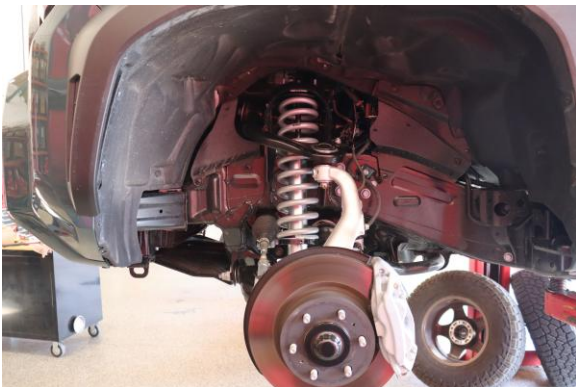
23. Install wheel and tire. Tighten lug nuts to manufacturer specification. Lower vehicle.
