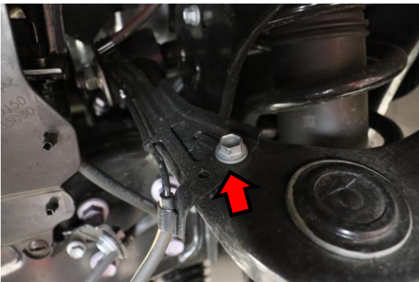
5. Remove the wheel speed sensor wire harness bracket from the upper control arm.
