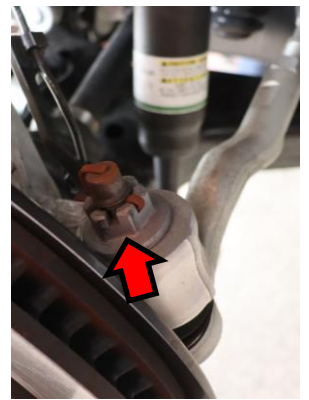
2. Remove cotter pins from the upper ball joint and outer tie rod end.
