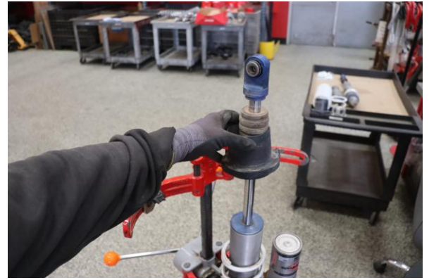
Step 8. Remove OE slider
