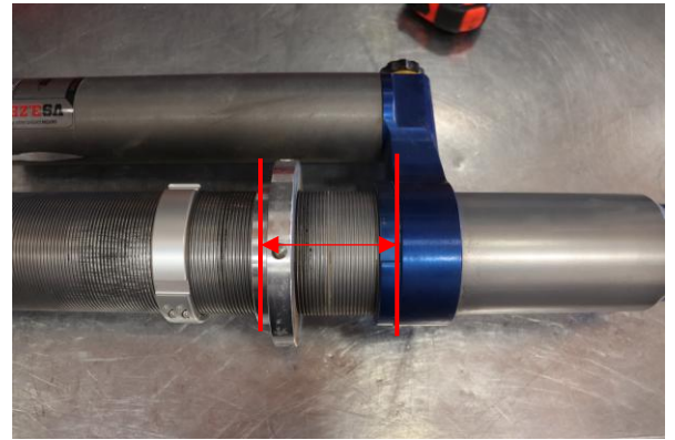
Step 10. Set pre-load to 50mm ( 2 in.) from bottom of spring seat to bottom of furthest point on reservoir bridge.
