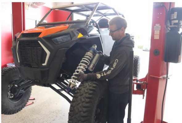
Step 5. Remove shock assembly from vehicle between upper and lower shock mounts.
