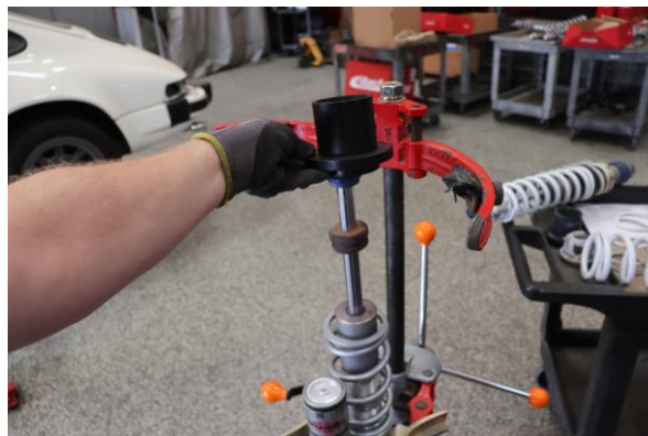
Step 14. Install Eibach spring slider 8001105 with larger face pointed away from secondary spring.
