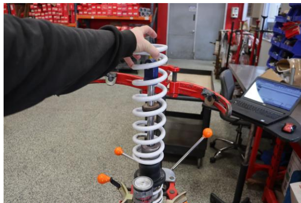
Step 8. Remove OE main spring.
