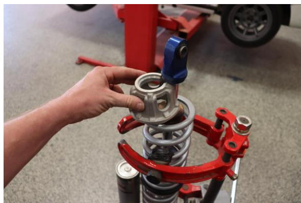
Step 16. Compress shock assembly enough to install lower spring retainer. Decompress shock and ensure spring and retainer sit flush on lower mount.
