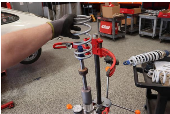
Step 13. Install Eibach secondary spring.
