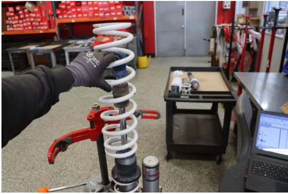
Step 7. Remove OE main spring
