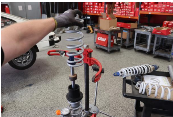
Step 15. Install Eibach main spring.
