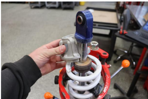
Step 7. Remove the spring retainer.
