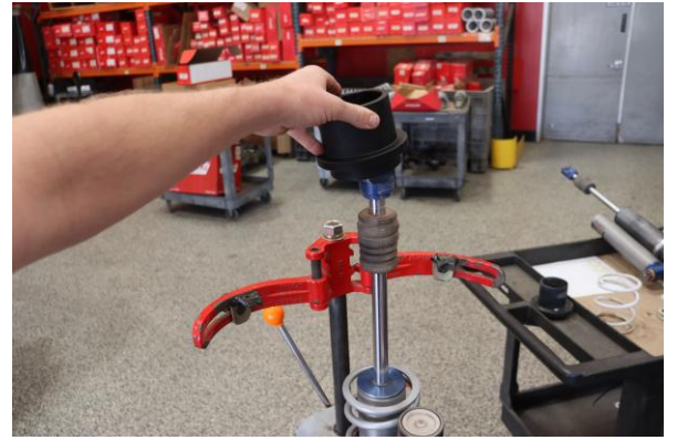
Step 14. Install Eibach supplied spring slider 8001498.
