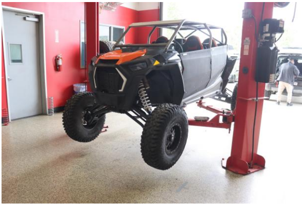
Step 1. Raise the front of the vehicle and support it with the proper safety equipment. Note: Never work on or under a vehicle that is not supported by the proper safety equipment.
