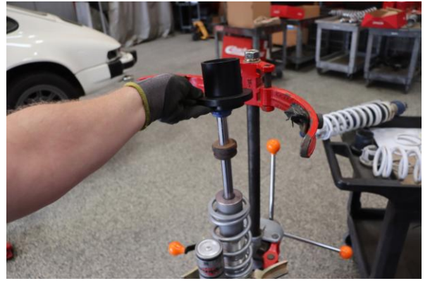
Step 14. Install Eibach spring slider 8001105 with larger face pointed away from secondary spring.
