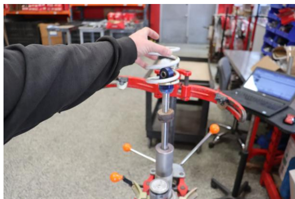
Step 10. Remove OE secondary spring.
