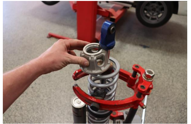
Step 16. Compress shock assembly enough to install lower spring retainer. Decompress shock and ensure spring and retainer sit flush on lower mount.
