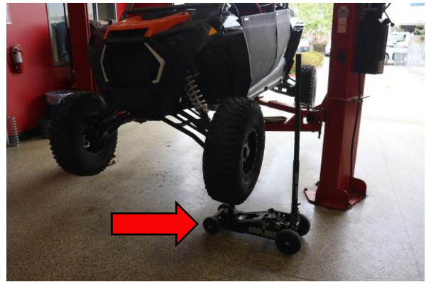
Step 2. Support the axle using a strap or jack to prevent axle damage.
