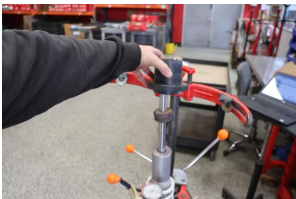
Step 9. Remove spring slider.
