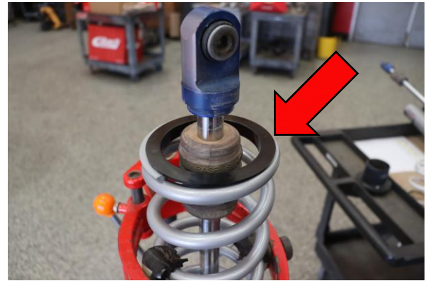
Step 16. Install ADAPTER350-375 on bottom of main spring.
