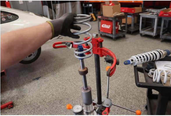
Step 13. Install Eibach secondary spring.
