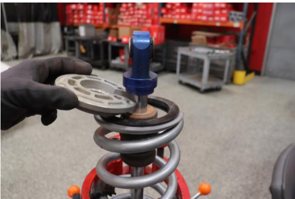
Step 17. Install lower spring retainer. Decompress spring assembly making sure that lower spring retainer and main spring sit flush with lower shock mount.
