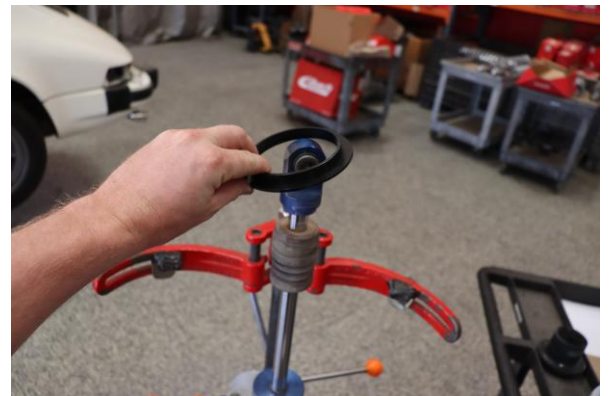
Step 12. Install ADAPTER350-375 on OE spring perch.
