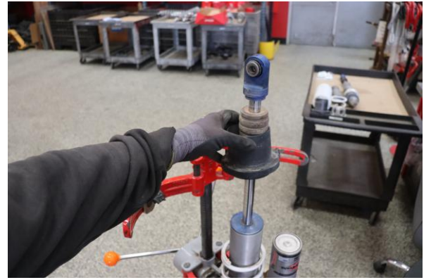
Step 8. Remove OE slider
