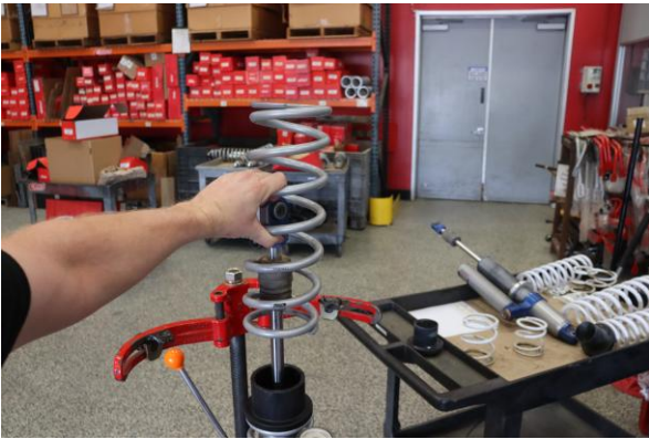
Step 15. Install Eibach main spring
