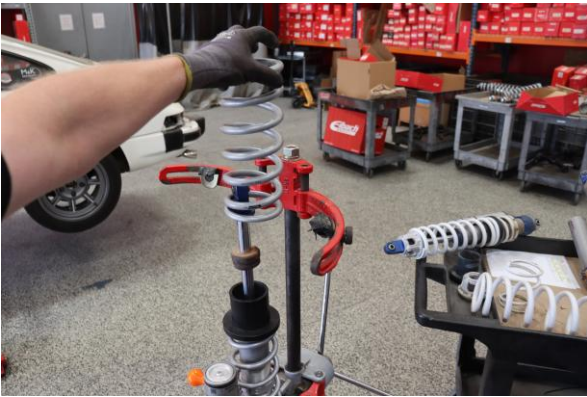
Step 15. Install Eibach main spring.
