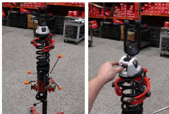
Step 10. Use a spring compressor to compress the spring assembly. Remove the lower spring perch.
