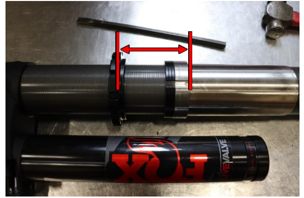
Step 14. Set crossover ring to 110mm (4 5/16in.) from bottom of spring seat to bottom of crossover ring.
