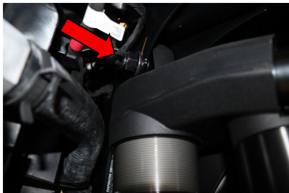
Step 7. Use two 21mm to remove the upper shock mounting nut and bolt.
