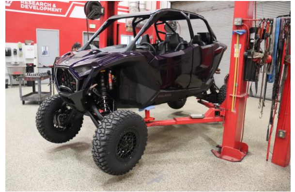
Step 2. Use a 19mm to remove both front wheels.
