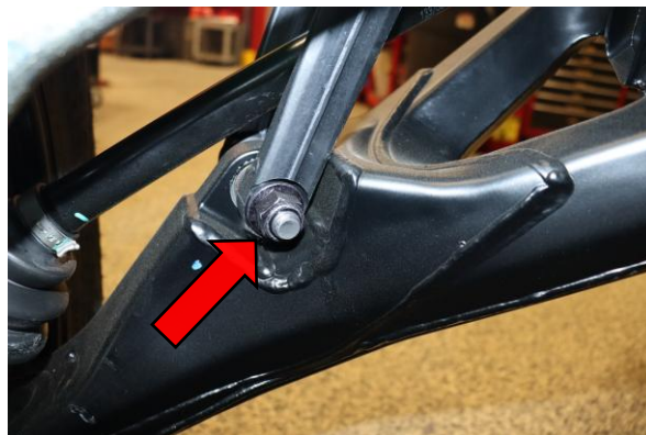
Step 8. Use two 21mm to remove the lower shock mount nut and bolt.
