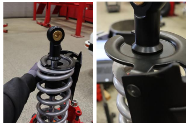
Step 18. Compress the spring assembly and install the lower spring perch. Decompress the spring assembly making sure that the lower spring perch seats fully against the lower shock mount.
