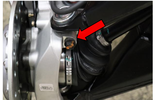
Step 4. Use a 15mm to remove the upper ball joint bolt.
