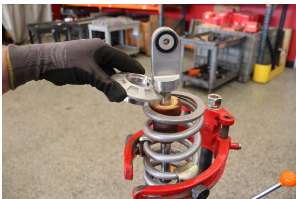
Step 17. Compress the spring assembly and re-install the spring retainer.
