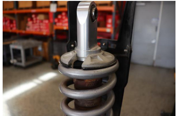
Step 22. Ensure spring and retainer sit flush on lower mount. Shown in photo above.
