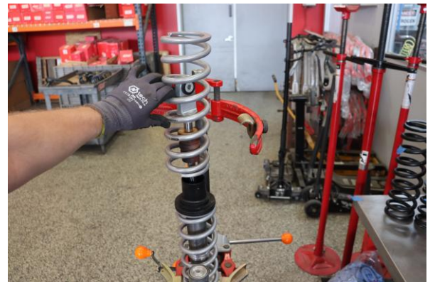
Step 16. Install Eibach main spring.
