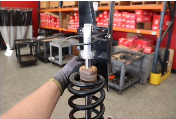
Step 9. Remove the shock guard.
