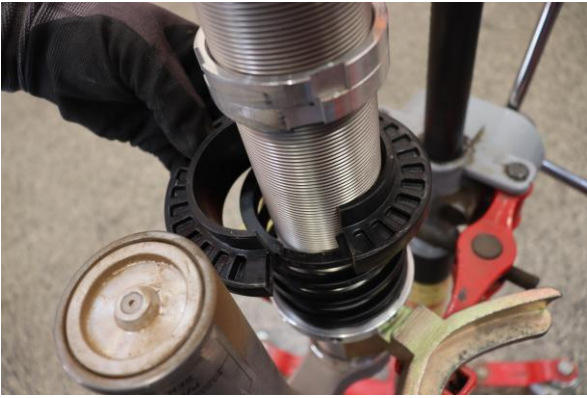
Step 13. Remove second OE spring slider.
