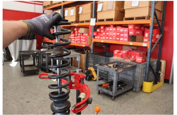
Step 10. Remove OE main spring.
