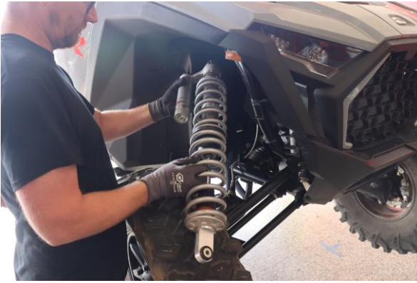
Step 19. Install shock into vehicle.
