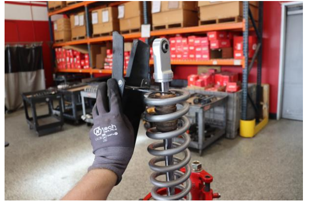
Step 20. Reinstall the shock guard.
