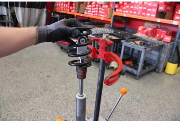
Step 11. Remove OE secondary spring.
