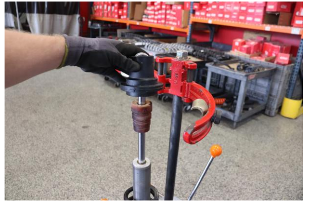
Step 10. Remove OE slider.
