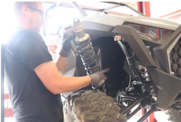
Step 5. Remove the shock for lower mount and then lower shock till it clears the plastic and remove shock upwards.
