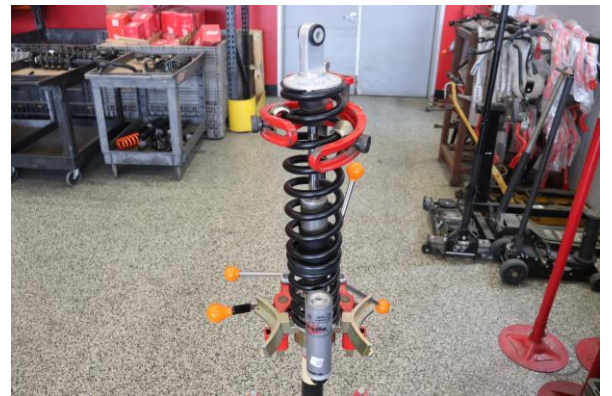
Step 6. Use spring compressor to compress shock assembly.
