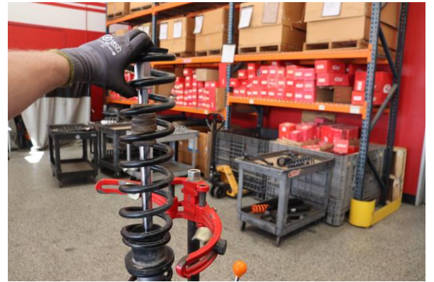
Step 10. Remove OE main spring.
