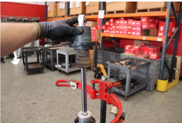
Step 11. Remove OE spring slider.
