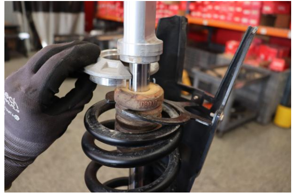
Step 8. Remove the lower spring retainer.
