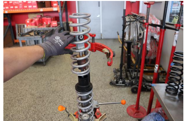
Step 16. Install Eibach main spring.
