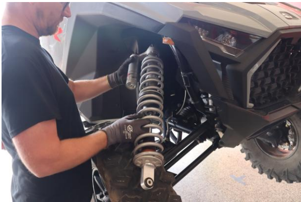
Step 19. Install shock into vehicle.
