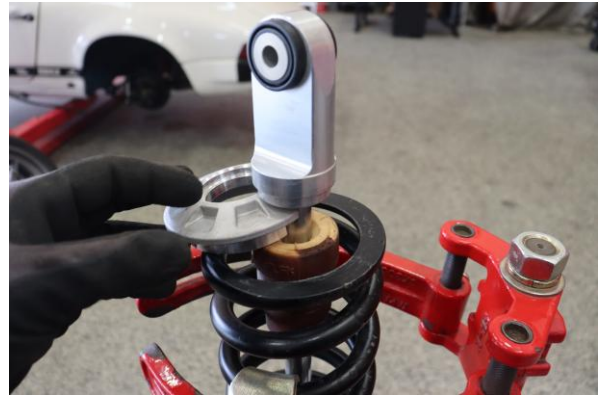
Step 8. Remove the lower spring perch.
