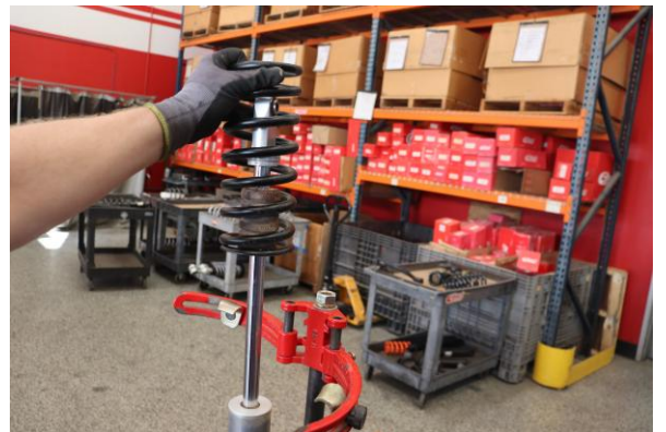
Step 12. Remove OE secondary spring.
