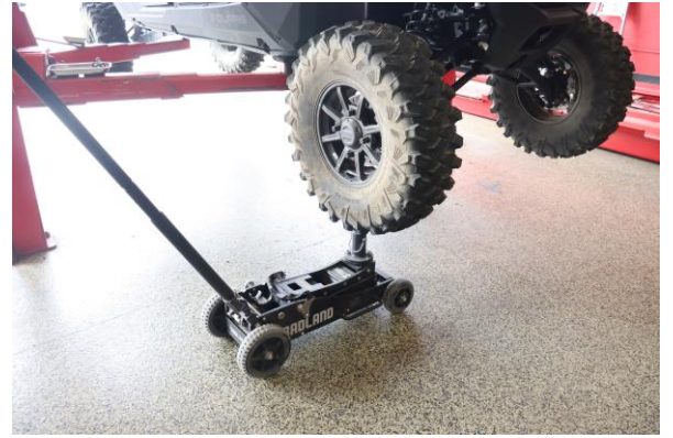
Step 2. Use a strap or jack to hold the suspension to prevent damage to axles.
