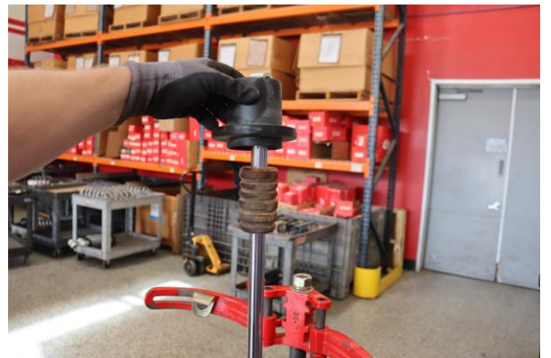
Step 18. Install Eibach supplied spring slider with larger face pointed away from secondary spring.
