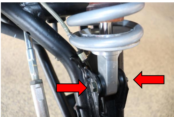
Step 21. Install lower shock bolt and tighten to manufacturer specification 44 ft-lb using 15mm socket and wrench.
