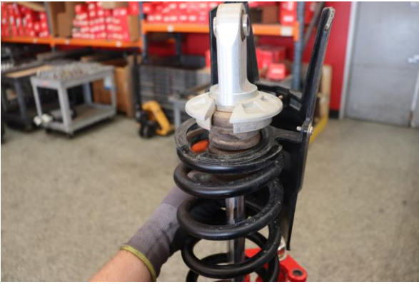
Step 7. Push the bump stop down to free lower spring perch from lower rod end mount.
