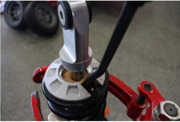
Step 7. Using a screwdriver or prybar push the bump stop away from the lower spring perch.
