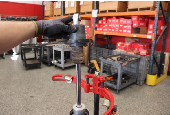
Step 11. Remove OE spring slider.
