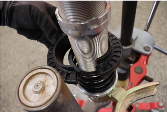
Step 13. Remove second OE spring slider.
