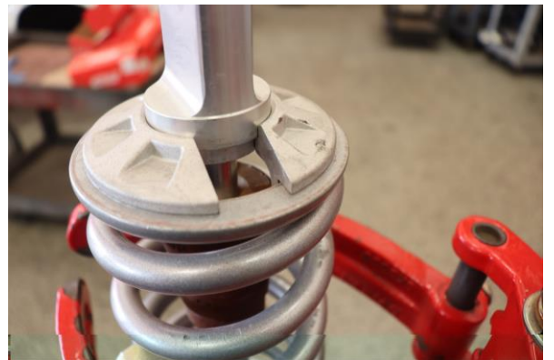
Step 18. Decompress shock and ensure spring and retainer sit flush on lower mount.
