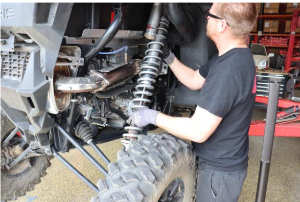
Step 23. Set shock assembly in vehicle by inserting top of assembly through opening in body panels and setting lower shock mount in trailing arm.
