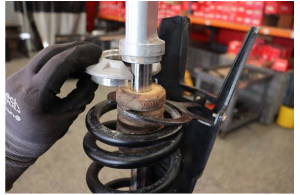
Step 8. Remove the lower spring retainer.
