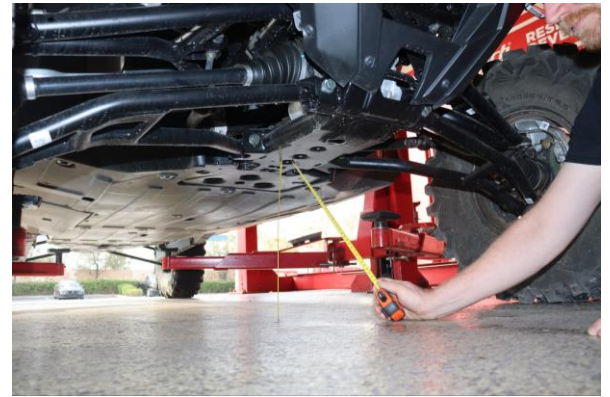
Step 22. Measurement shown from level floor surface to front skid plate 355mm (14" inches).
