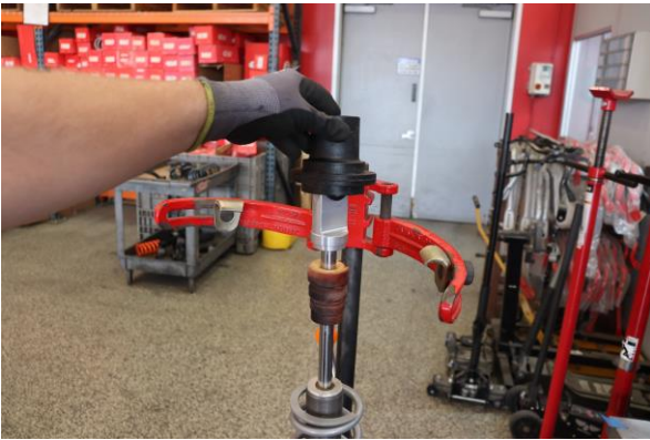
Step 15. Install Eibach spring slider with larger face pointed away from secondary spring.
