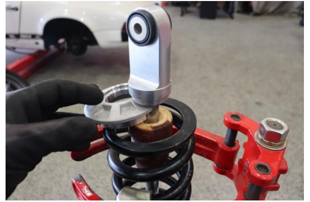
Step 8. Remove the lower spring perch.
