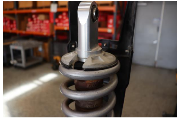
Step 22. Ensure spring and retainer sit flush on lower mount. Shown in photo above.
