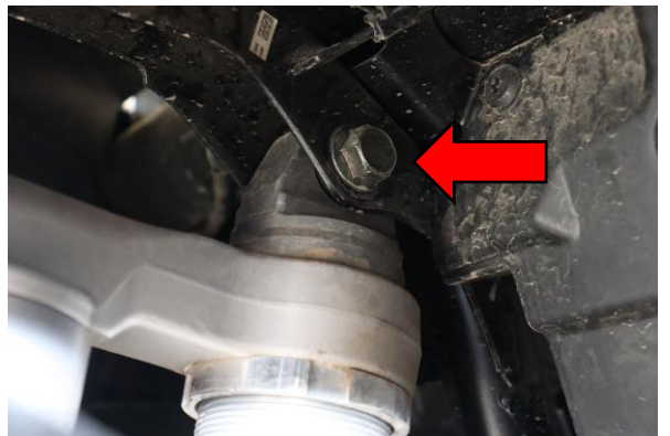
Step 24. Install upper shock mount nut and bolt. Tighten to manufacturer specification 74 FT-LB using 18mm wrench and socket.
