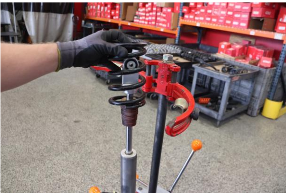
Step 11. Remove OE secondary spring.
