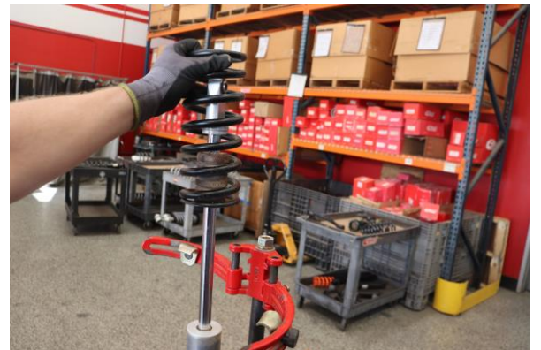
Step 12. Remove OE secondary spring.
