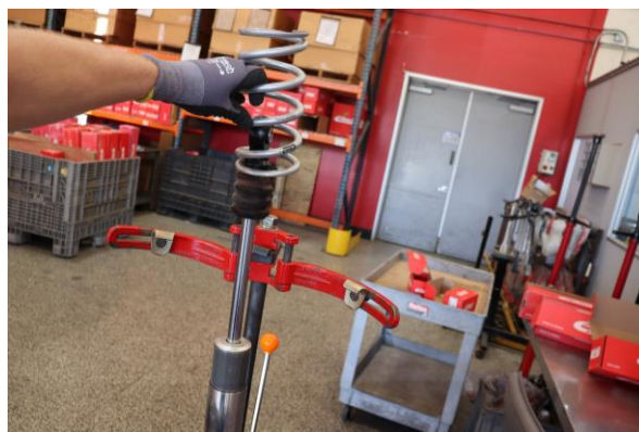
Step 16. Install Eibach front secondary spring.
