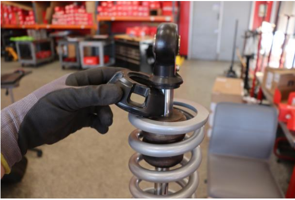
Step 19. Compress shock assembly enough to install lower spring retainer. Decompress shock and ensure spring and retainer sit flush on lower mount.
