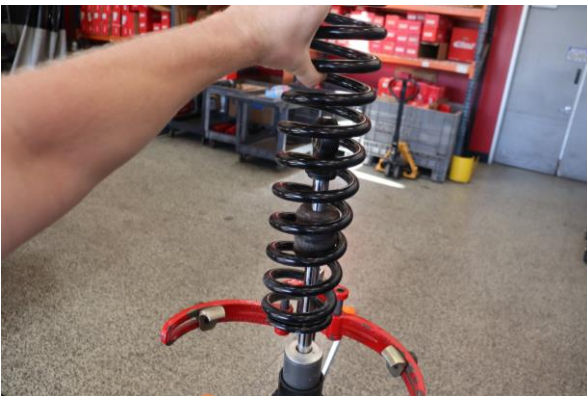
Step 11. Remove OE front main spring.
