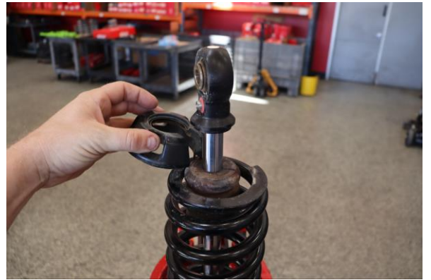
Step 10. Remove the lower spring retainer.
