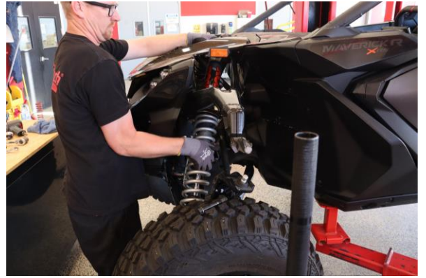
Step 20. Install shock in vehicle using upper mount bolt to hold assembly in place.
