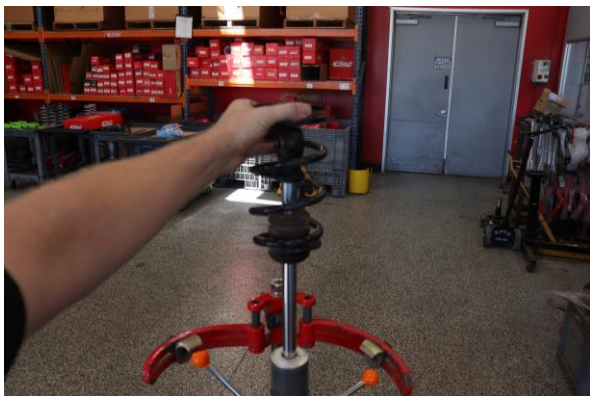
Step 13. Remove OE secondary spring.
