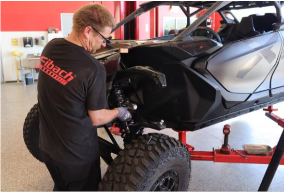
Step 7. Remove shock assembly from vehicle between upper and lower control arms.
