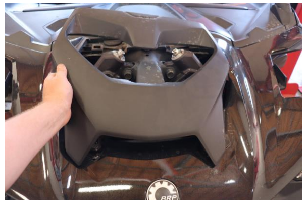
Step 24. Reinstall cover on front of car.
