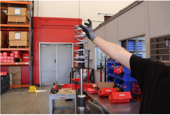
Step 13. Install Eibach secondary spring.
