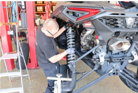
Step 17. Set shock assembly in vehicle by inserting top of assembly through opening in body panels and setting lower shock mount in trailing arm.
