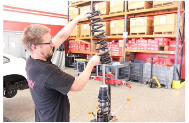
Step 8. Remove OE main spring.
