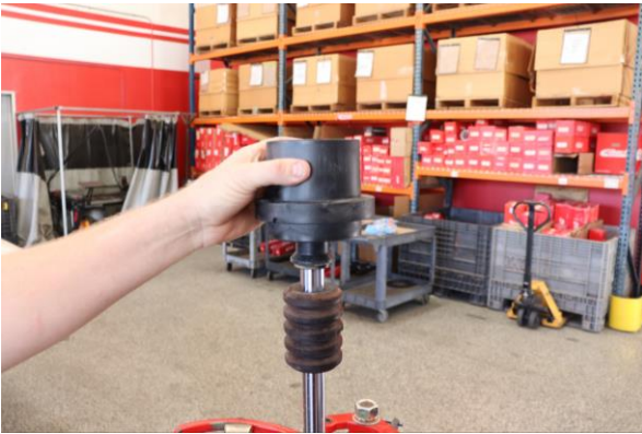
Step 9. Remove OE spring slider.
