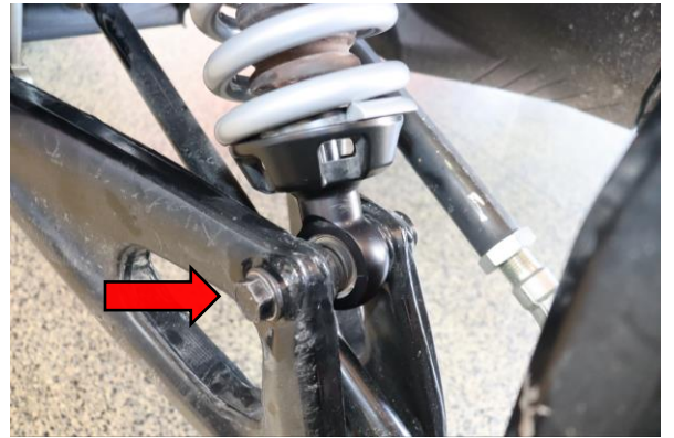
Step 22. Install lower shock bolt and tighten to manufacturer specification using 21mm socket.
