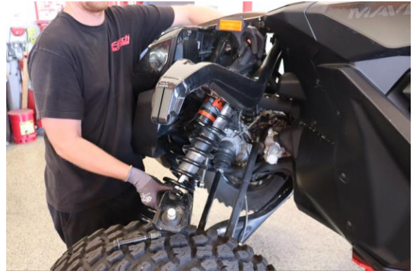
Step 8. Remove lower shock from mount first toward front of car.
