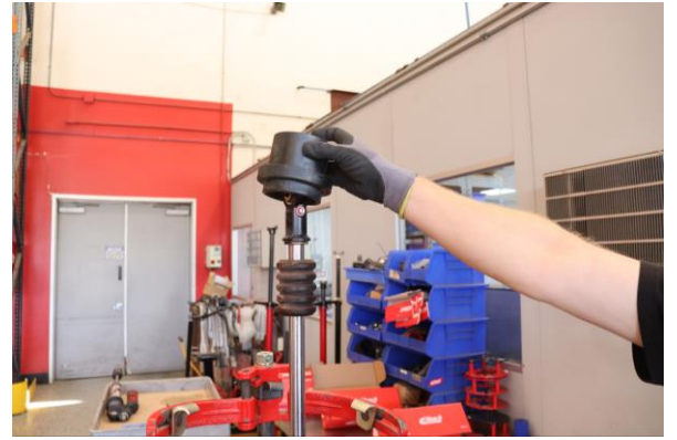
Step 14. Reinstall OE spring slider.
