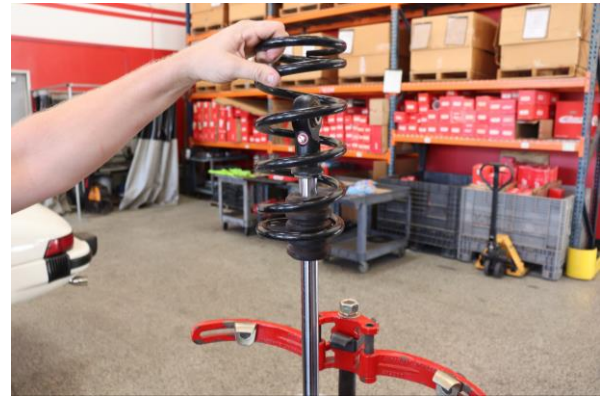
Step 10. Remove OE secondary spring.
