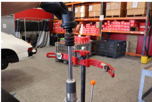
Step 17. Install OE spring slider with larger face pointed away from secondary spring.
