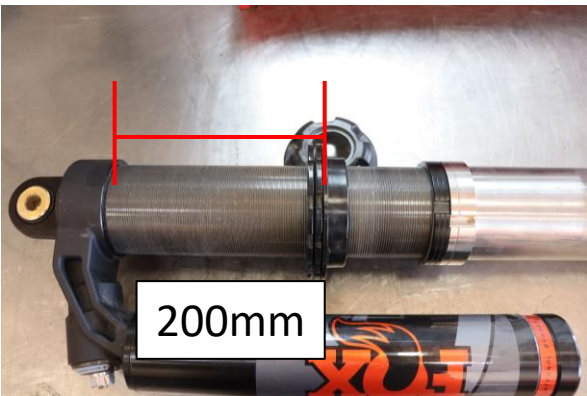
Step 11. Set pre-load to 200mm (7 7/8in.) from bottom of spring seat to bottom of furthest point on reservoir bridge. (Reservoir bridge is not flat relative to spring seat. Be sure to measure from the side opposite the reservoir).
