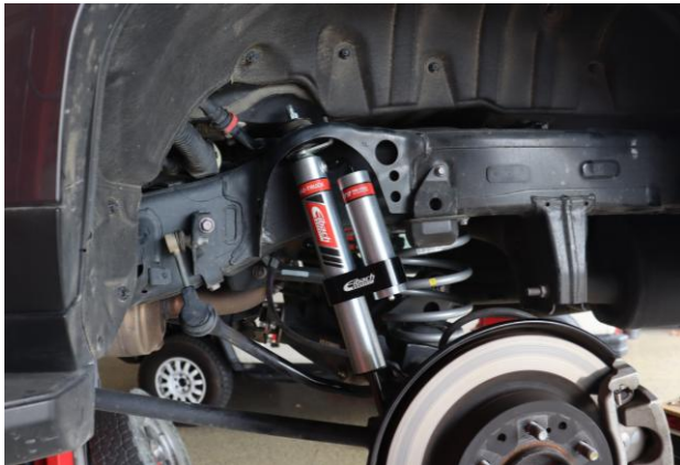
(LEFT SIDE) shown above with reservoir facing axle/rear of vehicle
