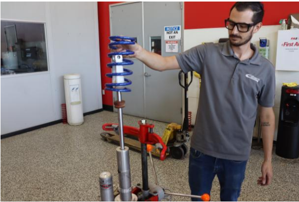
Remove the OE front tender spring.
