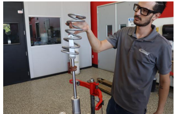
Install the Eibach Front Tender.
