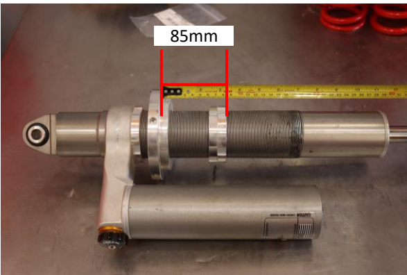
Set the crossover ring to 85mm (about 3 11/32") from the spring seat to the bottom of the crossover ring.
