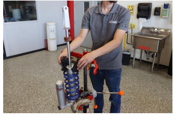
Remove the stock slider.
