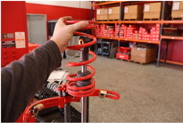
Step 31. Remove the OE rear tender spring.
