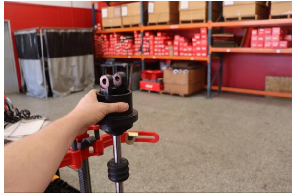
Step 14. Remove the oe slider.
