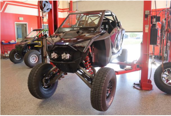
Step 1. Begin by jacking up the front of the vehicle.
