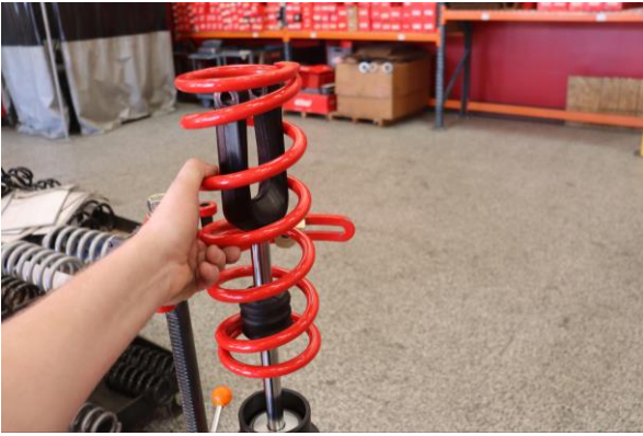
Step 13. Remove the OE main spring.
