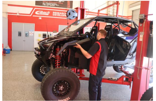
Step 4. Remove the fender.
