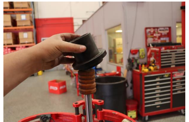
Step 18. Install Eibach spring slider with the short end facing the top of the shock.
