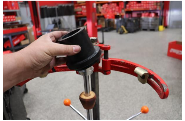
Step 14. Install Eibach front spring slider with the short end facing the top of the shock.
