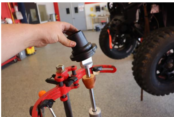
Step 9. Remove the OE spring slider.
