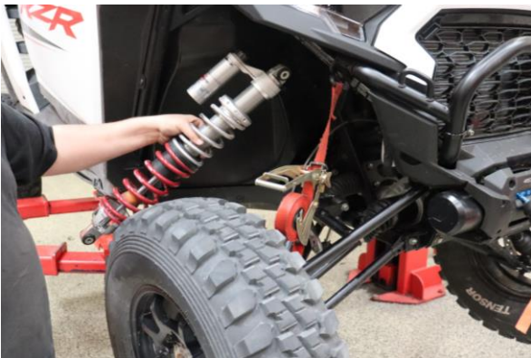
Step 17. Install shock assembly in the vehicle.
