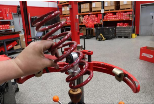
Step 15. Install Eibach main spring. Compress the spring assembly.
