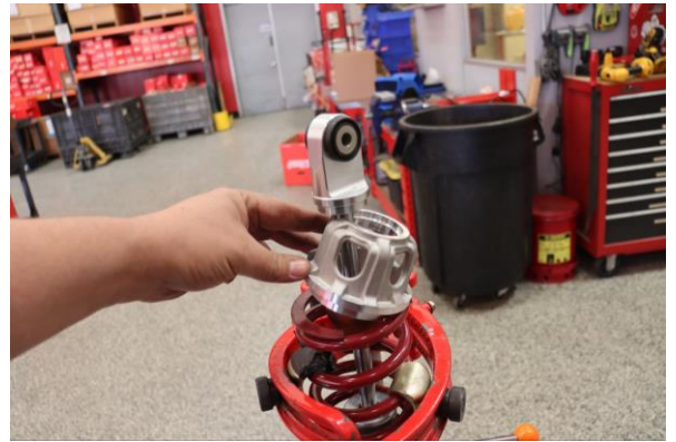
Step 16. Install OE lower spring perch. Decompress assembly and ensure lower spring perch engages lower shock mount fully.
