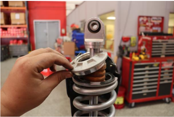
Step 21. Install the OE lower spring perch.
