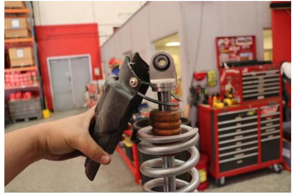
Step 20. Compress the spring assembly. Install the OE plastic shield facing away from the reservoir on the top of the assembly.
