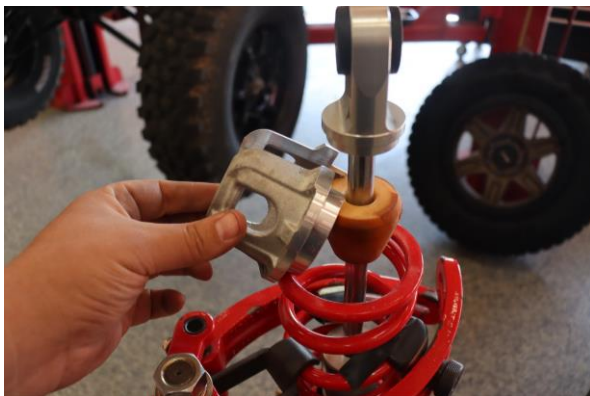
Step 7. Remove the lower spring perch. Decompress the spring assembly.
