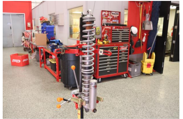
Step 22. Decompress the shock assembly ensuring the lower spring perch fully engages the lower shock mount and the plastic shield faces away from the shock reservoir.
