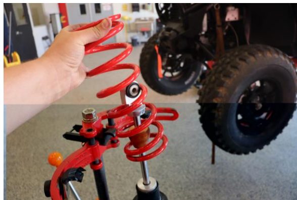
Step 8. Remove the OE main spring.
