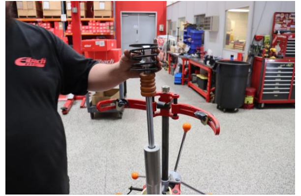
Step 14. Remove the second OE tender spring.
