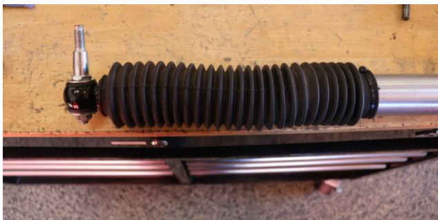
4. Install boot onto damper with included zip tie
