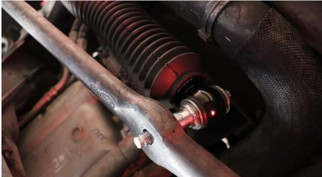
6. Install rod end of damper with stud into drag link, install M12 x 1.75 flange nut.
