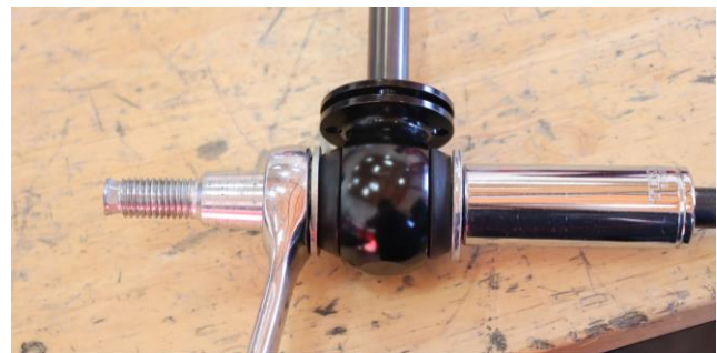
5. Install stud in rod end of steering damper using 22mm wrench and 19mm socket (may vary)
