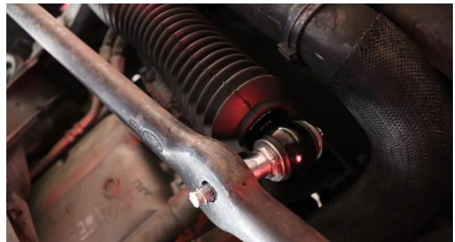
3. Remove damper stud from drag link using stud pulling tool & remove damper
