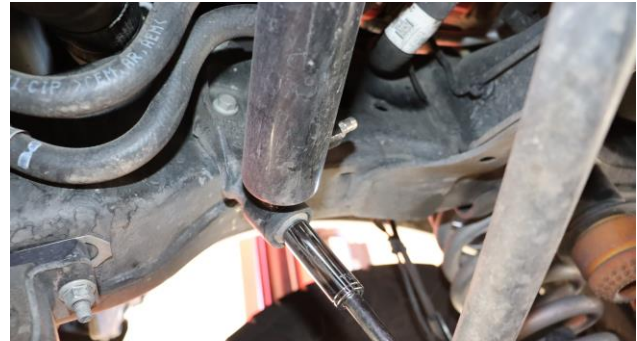
1. Remove 15mm bolt on right side of damper at frame
