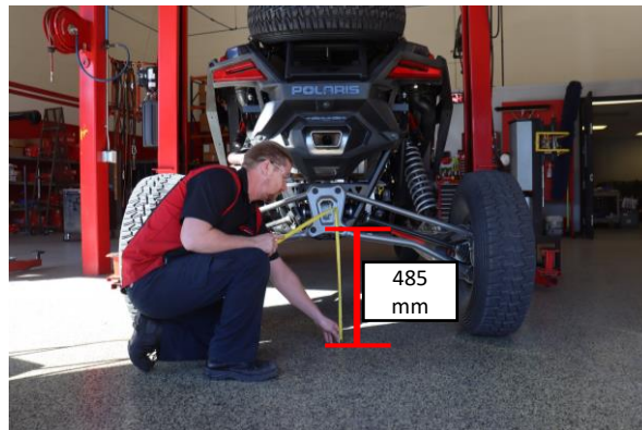
Step 39. Measure from the ground to the center of the lower radius arm bolt. The recommended preload measurement in Step 32 will get the vehicle close to the recommended ride height but each vehicle may vary some. As reference, skid plate measurement at recommended preload should be 406.4mm (16in.). We recommend setting the ride height at 485mm (19 3/32in.) measuring from the ground to the center of the lower radius arm bolt. Note: If you have larger than stock wheels and tires, the ride height will be increased. Due to the sensitivity of weight of these vehicles, weight distribution may change ride heights, additional pre-load may need to be added to compensate.
