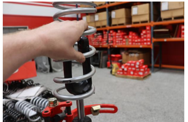
Step 18. Install the Eibach Front Tender.
