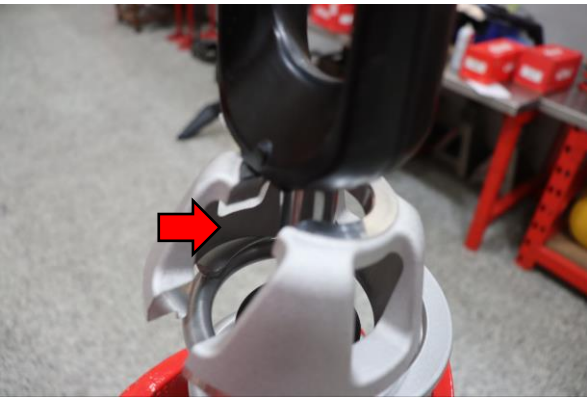
Step 20. Install the OE spring perch and ensure the boss on the clevis is aligned with the opening on the perch.
