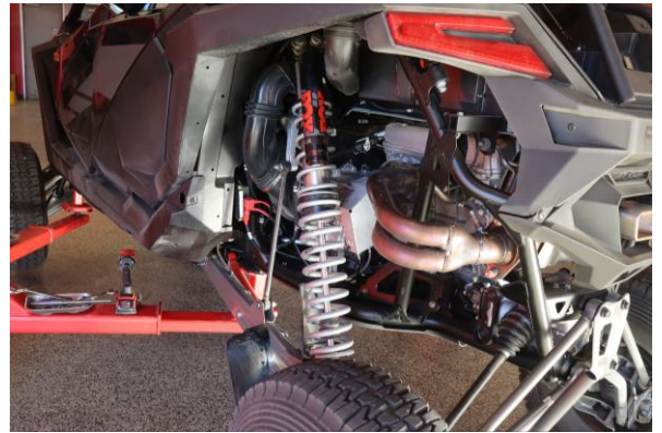
Step 38. Reinstall the shock. Reconnect the electrical connectors and top and bottom bolts and repeat on the opposite side.
