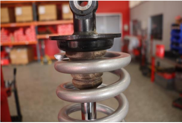
Step 5. Compress the coilover, then remove the spring retainer. Note: The bump stop will need to be pried down, out of the way of the spring retainer.
