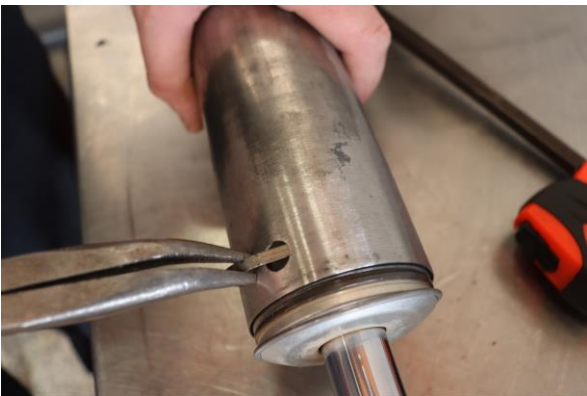
Remove the inner flat retaining wire through the access hole of the slider sleeve. Be sure not to distort or bend this wire as it will go back when finished.
