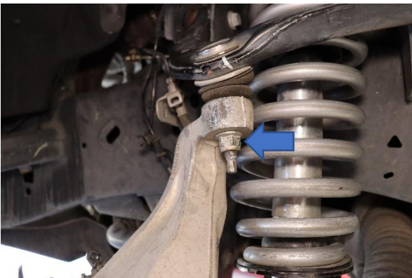
Step 4. Loosen the upper ball joint nut.
