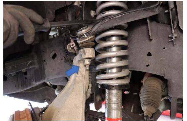
Step 15. Use a pry bar to ease the upper control arm down into the knuckle and fasten the nut on the bottom.
