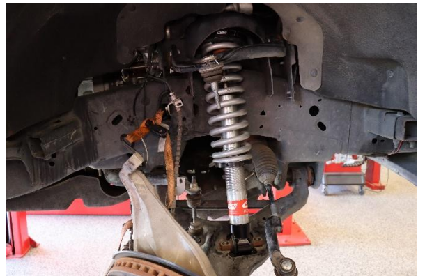
Step 11. Install new Eibach Coilover shocks
