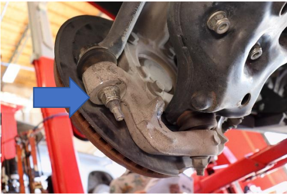
Step 3. Remove the tie-rod nut and disconnect the tie-rod from the knuckle
