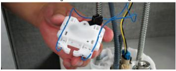
22. Install the sending unit onto the fuel pump module. Make sure the sending unit wires do not get pinched between the sending unit and the fuel pump module.
