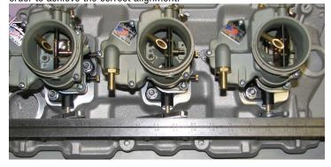
4. Once the correct angle and depth have been achieved, apply a small amount of Loctite to the small set screws and fully tighten them to secure the arms to the shafts. Twist each linkage to make sure that the arms will not slip on the shafts. It may be necessary to tighten the set screws several times before they bite into the throttle shafts and are locked in place.
