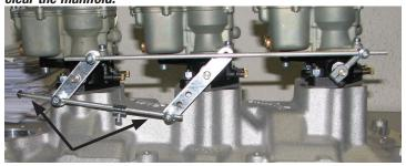
9. Twist the throttle arm on the center carburetor to wide open then inspect the other side to see that the pump cam is against the stop.
