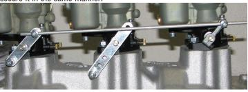
8. Install the capped rod, with the capped end forward, through the front and center carburetor swivel studs being sure to install the floating stop between. Leave roughly 1.5" between the rod cap and the front carburetor's swivel stud then tighten the swivel stud set screw on the center carburetor's throttle arm. Do not tighten the set screw on the floating stop at this time. *NOTE: Capped rod may require trimming to clear the manifold.*
