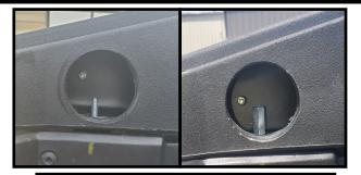
Re-attach the previously removed Washer and Coupling Nut to each of the 4 "Plug Inserts" and tighten with 3/8" wrench.
