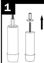
Remove: Washers and Coupling nuts from all 4 "Plug Inserts" and set aside. 2
