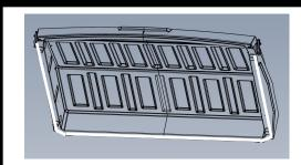
Apply included gasket to the outside edge of the rotokap base as shown.
