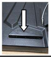
Plugs should be flush with the back panel of the tailgate (as shown below) if fully installed correctly.
