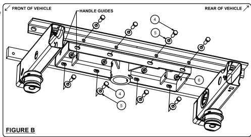
that the center ring protrudes through the bed floor. Maintaining the upward pressure from the lifting device onto the gooseneck hitch will ease the process of attaching the gooseneck center section to the crossarms. Remove lifting device before torquing hardware.
