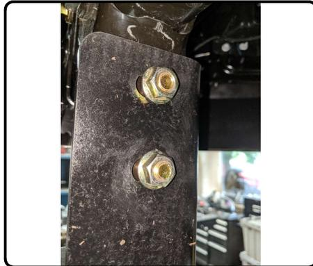
5. Torque 5/8" hardware to 159 ft-lbs, M12 hardware to 79 ft-lbs and 7/16" hardware to 70 ft-lbs.
