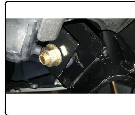
6. Torque all M10 fasteners to 48 ft-lbs, all M12 fasteners to 86 ft-lbs and all 5/8" fasteners to 180 ft-lbs.
