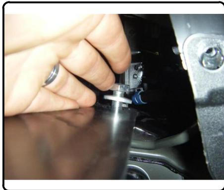
4. Loosely install M12 bolts with 1/2" conical tooth washers into existing weldnuts on the outsides of frame rails.
