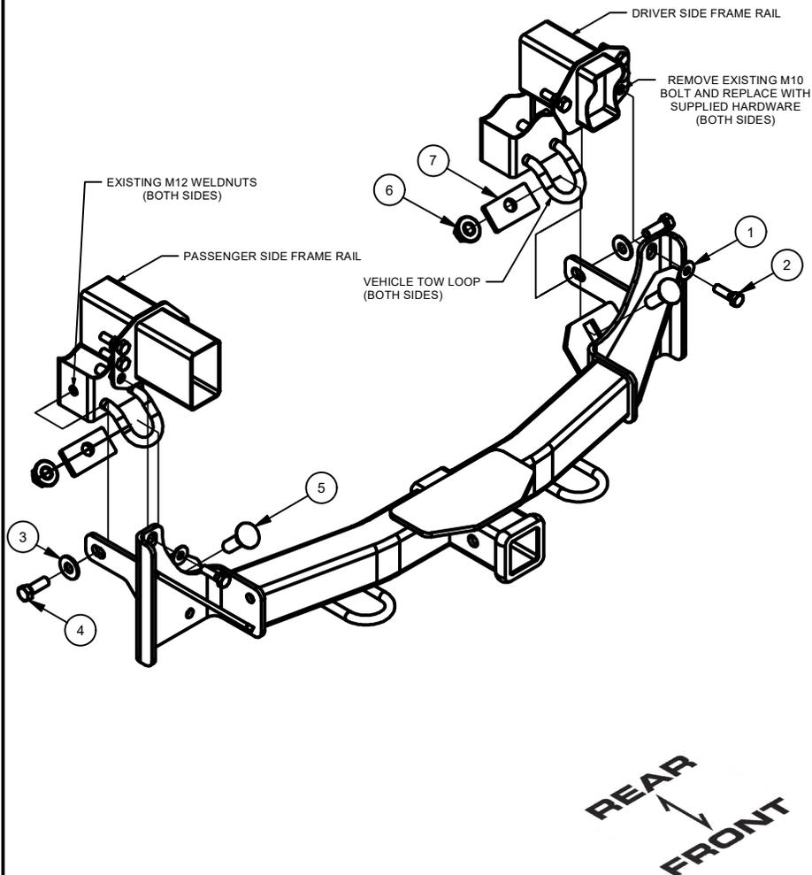
1. Remove one (1) hex bolt from the end of each frame rail with a 14mm socket (lowest outer bolt on each side) and return to vehicle owner. These will be replaced with the included M10 hardware.
