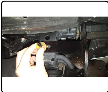
5. Insert 5/8" carriage bolts through the hitch mounting plates and tow loops. Secure hitch to tow loops by attaching supplied spacers and 5/8" flange nuts to carriage bolts.
