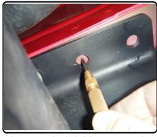
3. Remove M10 bolts, lower hitch and drill (4) holes at marked locations.
