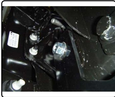
5. Fishwire 7/16 in. bolts and spacers into position and secure with nuts as shown.
