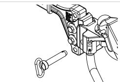
Snap-up one snap-up bracket at a time, ensuring that the clevis pin is installed before taking pressure off of the handle. Measure the front and rear bumper again. If you're within 1/2" of the measurement found at the top of step 5, no further adjustment is needed.
