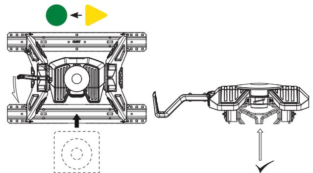
If the kingpin is resting on top of the jaws, immediately lower the trailer jacks to lift the kingpin off the jaws. Inspect the 5th wheel for damage that may have resulted from the improper coupling attempt. Under no circumstances should the 5th wheel unit be used if damage exists. If no damage exists, review coupling instructions and repeat procedure.
