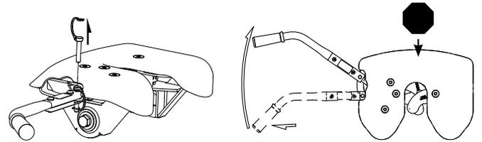
**NOTE:** If the operating handle fails to latch in the unlock position while the kingpin is in the jaws, refer to steps 1, 2 and 5 in the 'Preparation Troubleshooting' section on page 6. Never attempt to uncouple without the handle being in the unlocked position.
