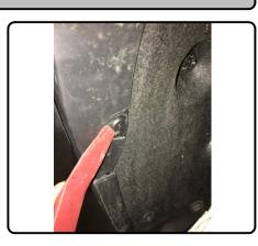
4. Remove (2) fasteners from each side of bumper cover using 8 mm socket which are now accessible due to wheel well trim removal.
