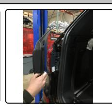
6. Located in trunk of vehicle remove interior panel to access tail light and remove exposed fastener using 10mm socket.
