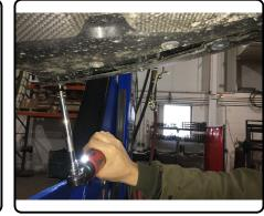
3. Remove (3) rivets from wheel well trim above each tire. To remove rivets push small center rod through rivet with a small punch. Pry rivets from trim.
