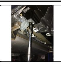
12. Raise hitch and bumper beam into position onto vehicle studs and secure using exisitng vehicle hardware. Use vehicle hardware to reattach driver side hanger bracket. Use hanger on hitch to reattach passenger side exhaust. <a href="MOTE"><u>NOTE</u>: Remove driver side exhaust bracket stud and replace with provided M8 hardware.</a>
