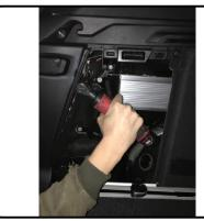
7. Remove (2) nuts from each tail light using 10mm socket.
