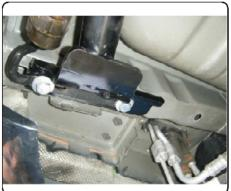
6. Torque all M12 fasteners to 86 ft. lbs. Raise exhaust back into position.
