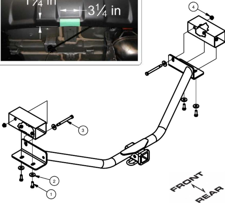
1. Lower exhaust by removing (3) rubber isolators. To ease installation, lower and remove spare tire temporarily.
