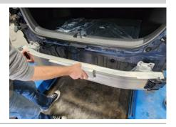
Push the thin metal piece under the bumper plate inward and make it flush with the end panel on each side.
