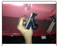
4. Raise hitch into position, feeding ends of fishwires through mounting holes on the hitch frame brackets. Using attached fishwires, pull bolts through holes in side of frame rails and hitch frame brackets. Secure with (8) 7/16" flange nut, as shown.
