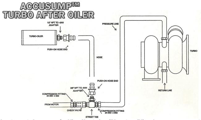
Locate your turbo pressure feed line. Your turbo will have two oil lines (one pressure, one return). The pressure line enters the top of the turbo, with the return line exiting the bottom.
