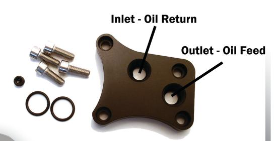
Note: We included a 1/8" NPT port to allow for installation of an oil temperature or oil pressure sensor. If you do not wish to use this port be sure to install the provided plug using thread sealing tape.
