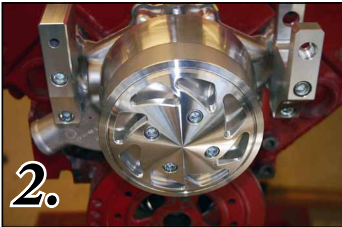
Photo-2 Install The Water Pump Pulley (6267-A) and the Water Pump Cap (331-A) using (4) \frac{5}{16} x \frac{7}{8} " Long Fine Thread SHCS (S186) as shown.
