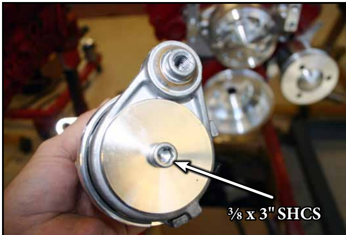
Photo-8 1. Hold Tensioner Body in a vise to remove bolt & washer from tensioner pulley. Note: Bolt is a left handed thread, turn clockwise to remove. Install the Tensioner into the 20256-B Bracket cover use a \frac{3}{8} x 3\frac{1}{4} " SHCS and install the (781-A) cover as shown and bolt into place.
