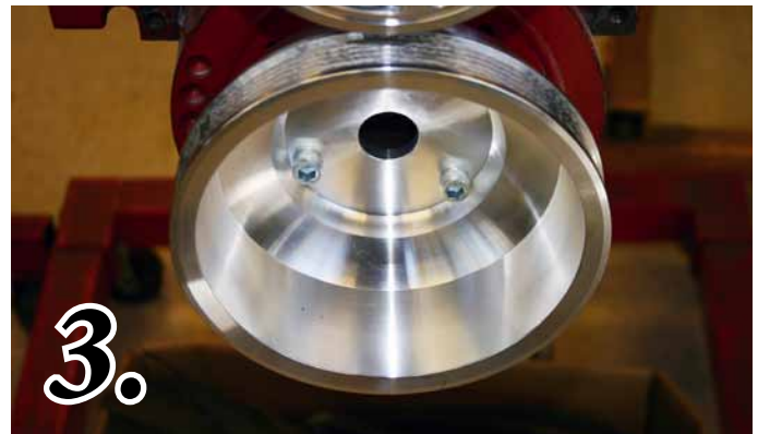
Photo-5 Install the Power Steering pulley (619-A) to the Remote Power Pump (Press Fit) and (740-A) Cover.
