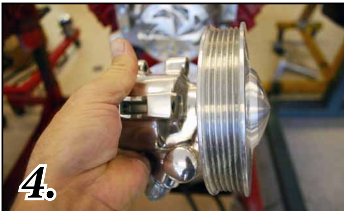
Photo-2 Install The Water Pump Pulley (6267-A) and the Water Pump Cap (331-A) using (4) \frac{5}{16} x \frac{7}{8} " Long Fine Thread SHCS (S186) as shown.
