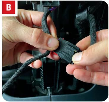
**STEP 5:** Route the Data Wiring Harness along factory wiring to the driver side kick panel area **(A)**. Using the supplied zip ties, secure the Harness to the factory wiring **(B)**.
