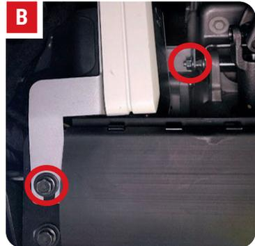
**STEP 2:** With the DSP/Amplifier Unit now mounted in place, locate and remove a 10mm bolt from the factory ground point above the driver side kick panel **(A)**. Install the terminal end of the Ground Cable on to the factory ground point being sure to not leave off the factory ground wire **(B)**. Using the supplied zip ties, secure any installed wires up and out of the way.
