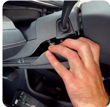
**STEP 4:** With the bottom steering wheel cover removed, locate the 8 pin factory connector on the bottom side of the steering wheel and disconnect it **(A)**. Install the t-harness end of the Data Wiring Harness in-line with the factory connector **(B)**.
