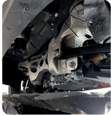
**STEP 2:** Next, remove the factory alert speaker. Remove the two 10mm bolts holding the factory alert speaker to the under body of the vehicle. Unplug the speaker and set aside.
