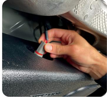
**STEP11:** Finally, remove two #2 phillips screws from the under body panel that was removed from the underside of the vehicle. Install the two Borla Speaker Grills (BOR-FME21G) and secure them to the panel using the previously removed phillips screws.
