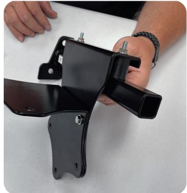
**STEP 6:** With the passenger side bracket assembled, begin assembling the driver side bracket by attaching the remaining two rubber isolators to bracket "1" using two of the 10mm nuts. Next, attach bracket "1" with the rubber isolators to bracket "3" using two 10mm nuts.
