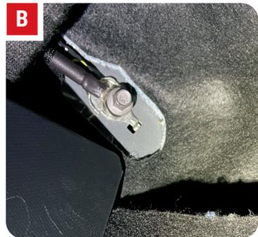
**STEP 3:** To complete the installation, install the supplied fuse into the fuse holder on P-BOR-PWR-HAR that was previously installed near the battery. Proceed with testing the system for functionality and putting the vehicle back together.
