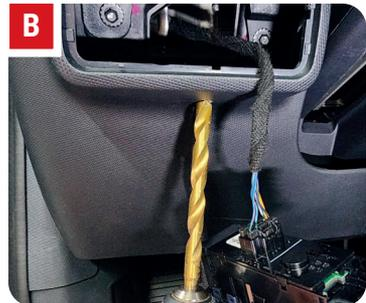
**STEP 2:** Feed the 4 pin connector end through the 1/2 inch hole and pull through (A). Then, using a wire snake or similar, route the 4 pin connector end down to the driver side kick panel area (B).
