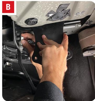
**STEP 8:** With the brackets installed, next move on to routing the Speaker Wiring Harness (BOR-FMESP-K-HAR) into the area exposed by removing the under body panel. Begin from the inside of the vehicle and pull back the carpet in the trunk to expose the rubber grommet in the driver side rear corner (A). Remove the factory grommet and route the enclosure connector down through the opening to the underside of the vehicle until the pre-installed grommet can be seated in place (B).
