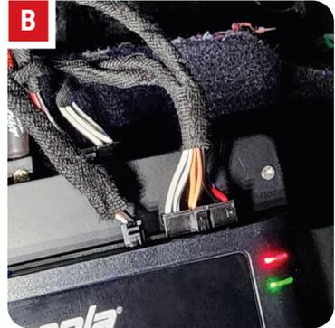
**STEP 5:** Finally, connect the 2 pin white connector from the Data Wiring Harness to the previously ran Speaker Wiring Harness in the driver side kick panel area.
