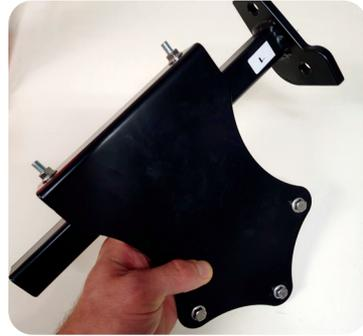
**STEP 7:** Install the two bracket assemblies onto the vehicle. Bracket "2/4/5" installs on the passenger side of the vehicle. Use the original 15mm bumper bolts that were previously removed to secure the assembly into place **(A)**. Bracket assembly "1/3" installs on the driver side of the vehicle. Use the original 15mm bumper bolts that were previously removed to mount the bracket into place **(B)**.
