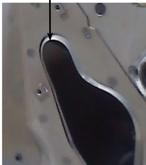
Radius may need to be trimmed for plate to sit flush.
