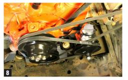
Typically, the adjusting arm will mount off the "lower" water pump bolt (especially to allow space for generator/alternator bracket arm); however, in some cases the upper location can be used. (Figs. 6-7)
