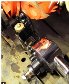
Loosely install the power steering pump (the open hooked end attaches to the lower rear stud on the pump, while the front bolts directly to pump as illustrated in Fig. 4).
