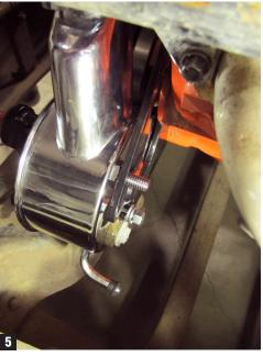
4. Loosely attach the adjusting arm bracket to the front of the pump and the engine. For "short" water pump applications, the dogleg points towards the pump; for "long" water pump applications, the dogleg in the bracket goes towards the engine. (Fig. 5)
