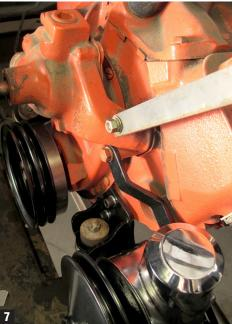
Verify the fit of your belts with the bracket positions; generally, a 15466 sized V-belt works best with a #CP38810 (PS pump), #CP38813 (dual-groove water pump), and #CP38811 crank pulley configuration. Tighten all bolts/nuts and adjust the belt tension as normal. (Fig. 8)
