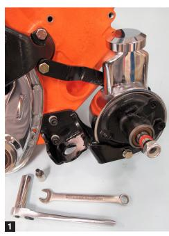
2. Unbolt stock bracket: replace with #PS808 using supplied cap screw Allens and lock washers. Install new motor mounts at this time if necessary. (Fig. 3)
